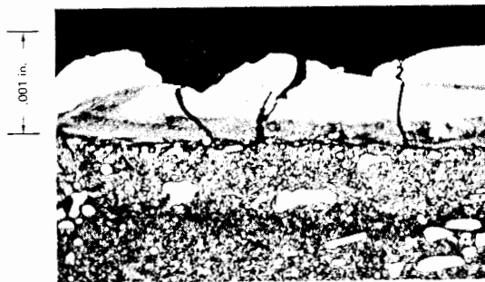
Fig. 6b. EDM on D2 tool steel, 61 R_c , redeposited metal on surface.
