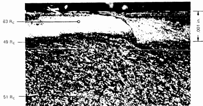
Fig. 6a. Drilling 4340, 51 R_c , with dull drill white (untempered martensite) layer.
