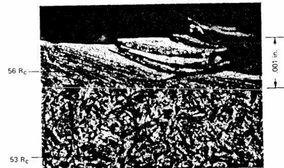
Fig. 6c. Reaming 4340, 53 R_c , with dull reamer tears from built-up edge.
