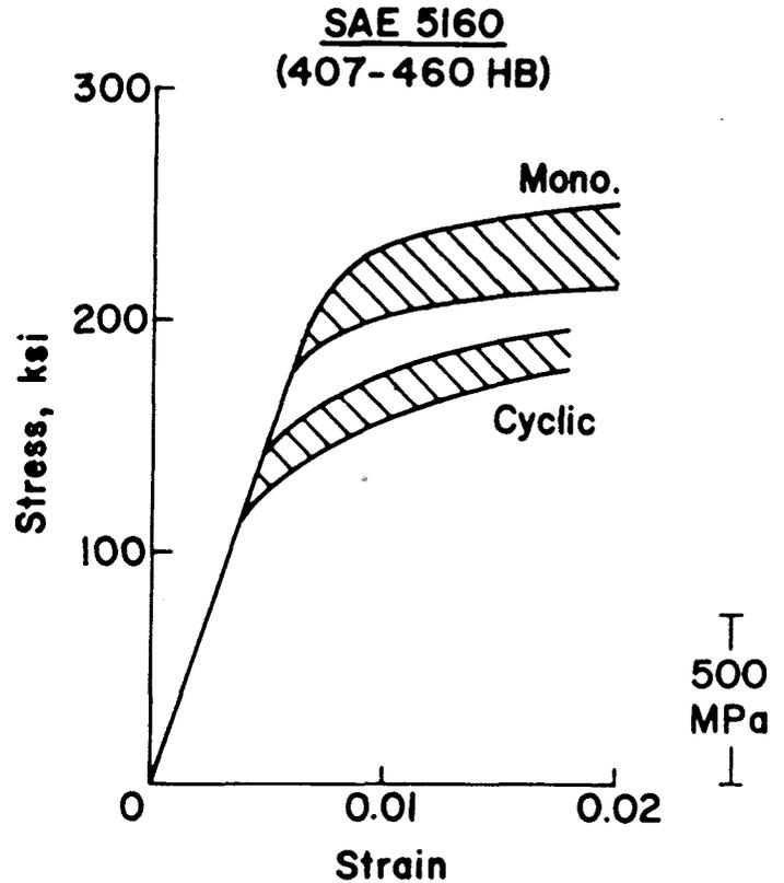
Fig. 4 - Monotonic and cyclic stress-strain curves for SAE 5160 spring steel
