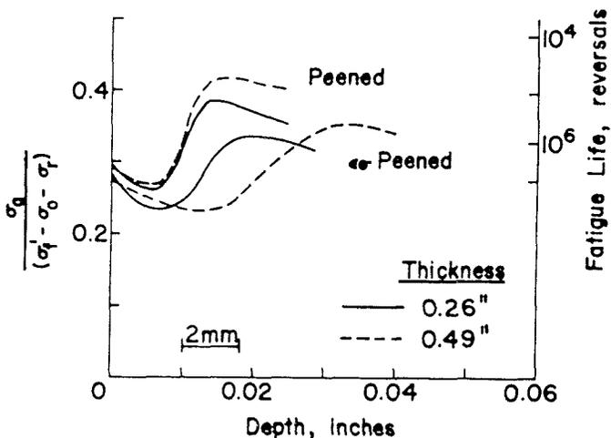
Fig. 16 - Stress parameter profiles for predicting failure location and lifetime
