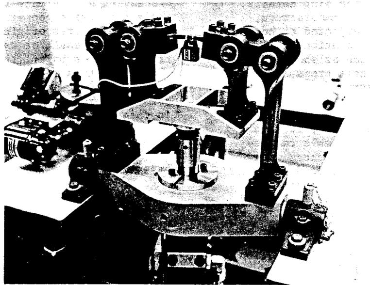
Fig. 3 - Four-point bending apparatus installed on servo-hydraulic actuator
