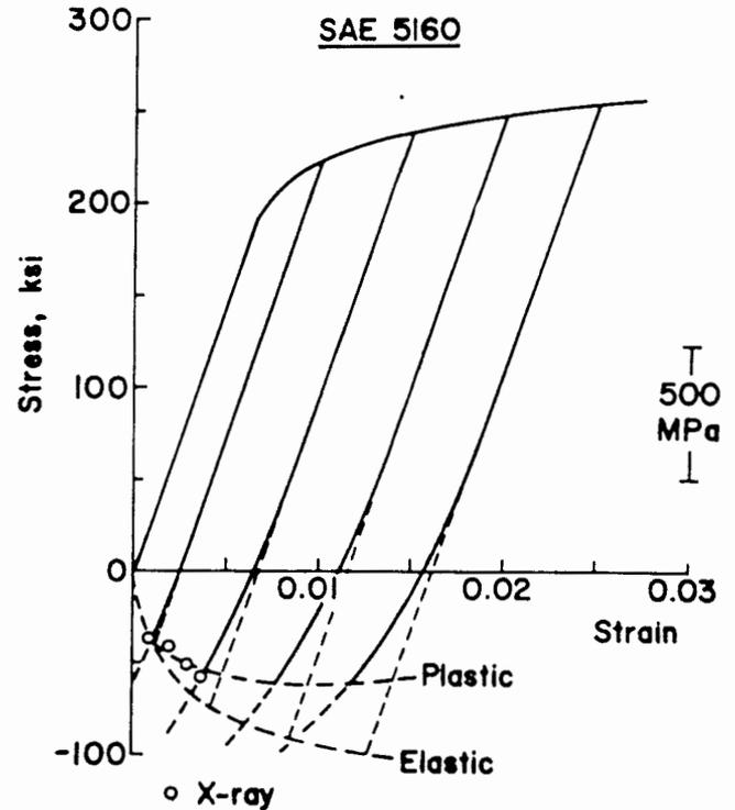
Fig. 11 - Procedure for determining residual stresses resulting from bending prestrains
