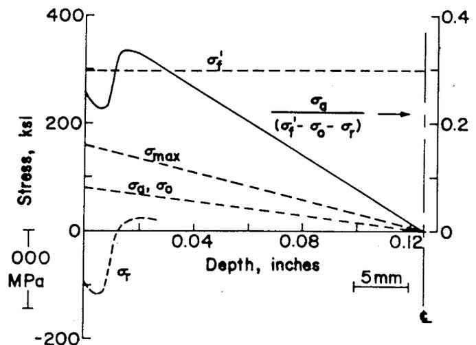
Fig. 15 - Procedure for performing fatigue analysis of a peened bending member
