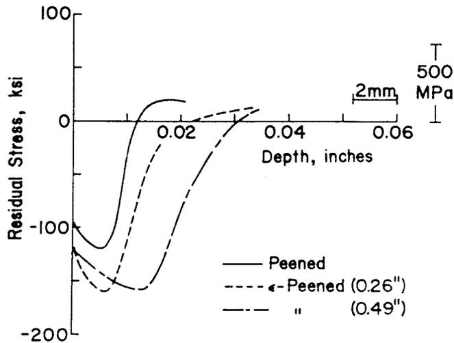
Fig. 13 - Residual stress profiles obtained with various peening operations
