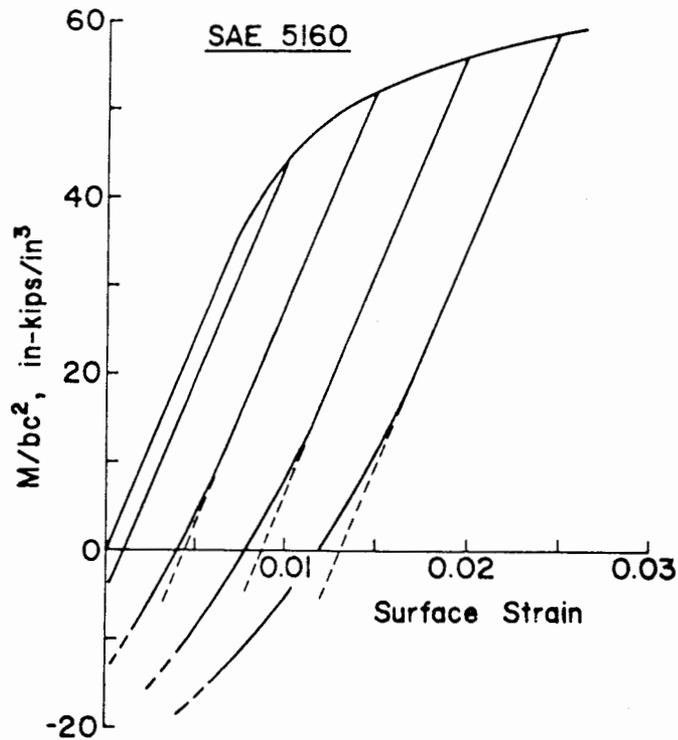
Fig. 10 - Procedure for determining residual surface strains resulting from bending prestrains
