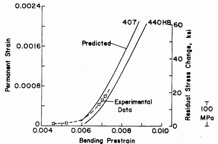
Fig. 12 - Comparison of predicted and experimental permanent strains resulting from bending prestrains
