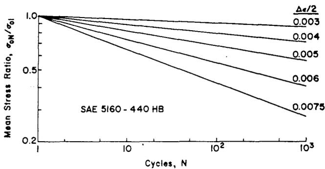
Fig. 8 - Representation of mean stress relaxation rates for various strain amplitudes
