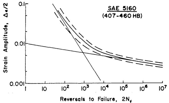
Fig. 5 - Strain-life curve for SAE 5160 spring steel. Dashed band indicates 95% confidence interval
