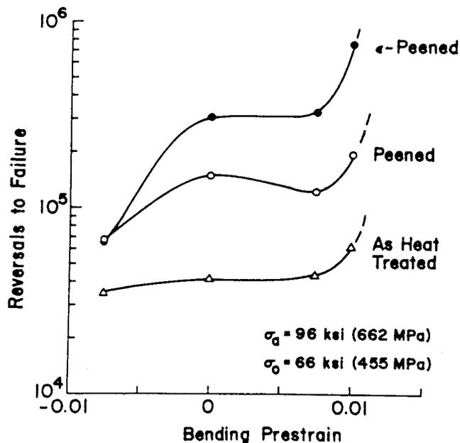
Fig. 14 - Fatigue lives of bending members subjected to various processing sequences
