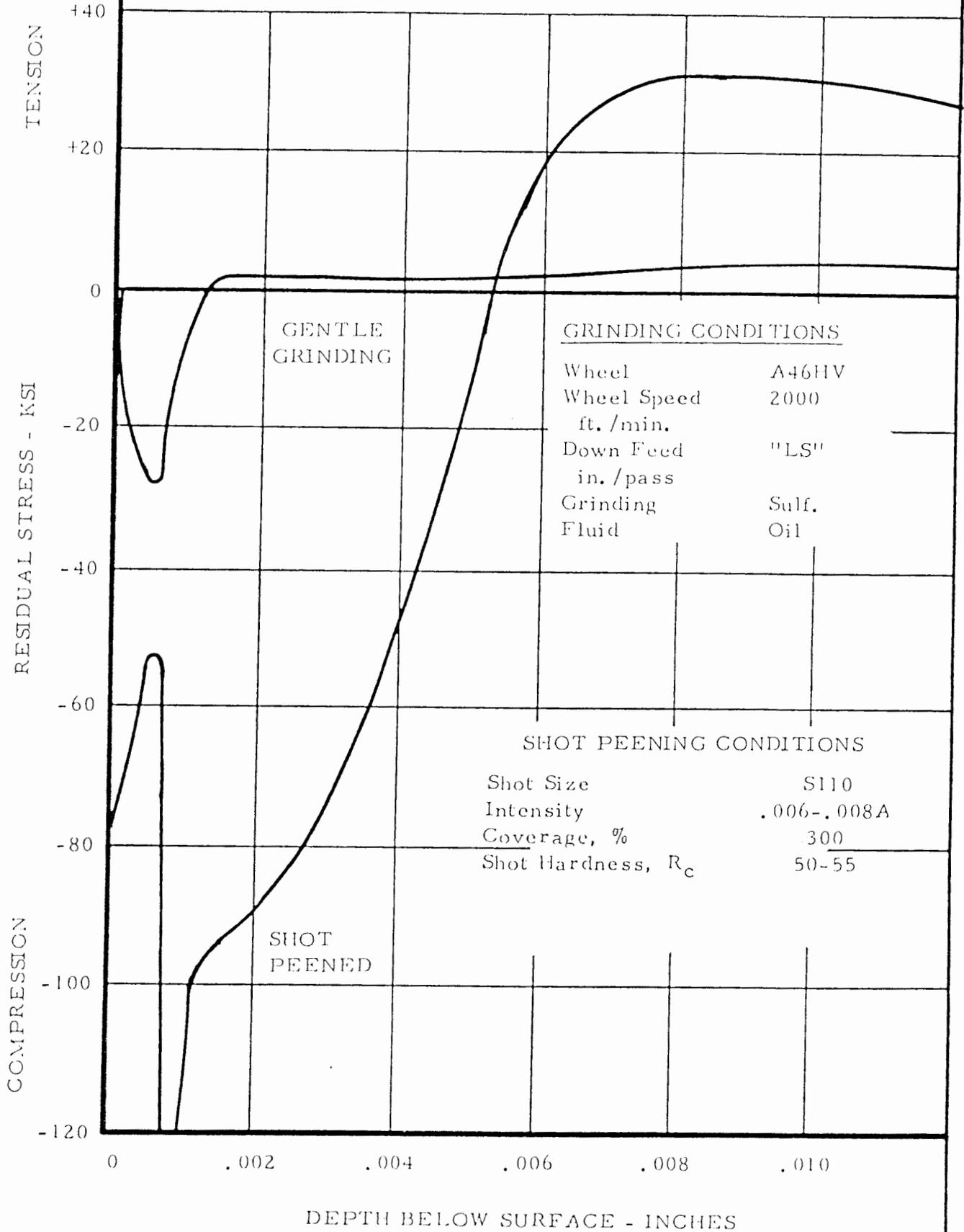
FIGURE 2. Residual Stress vs. Depth
