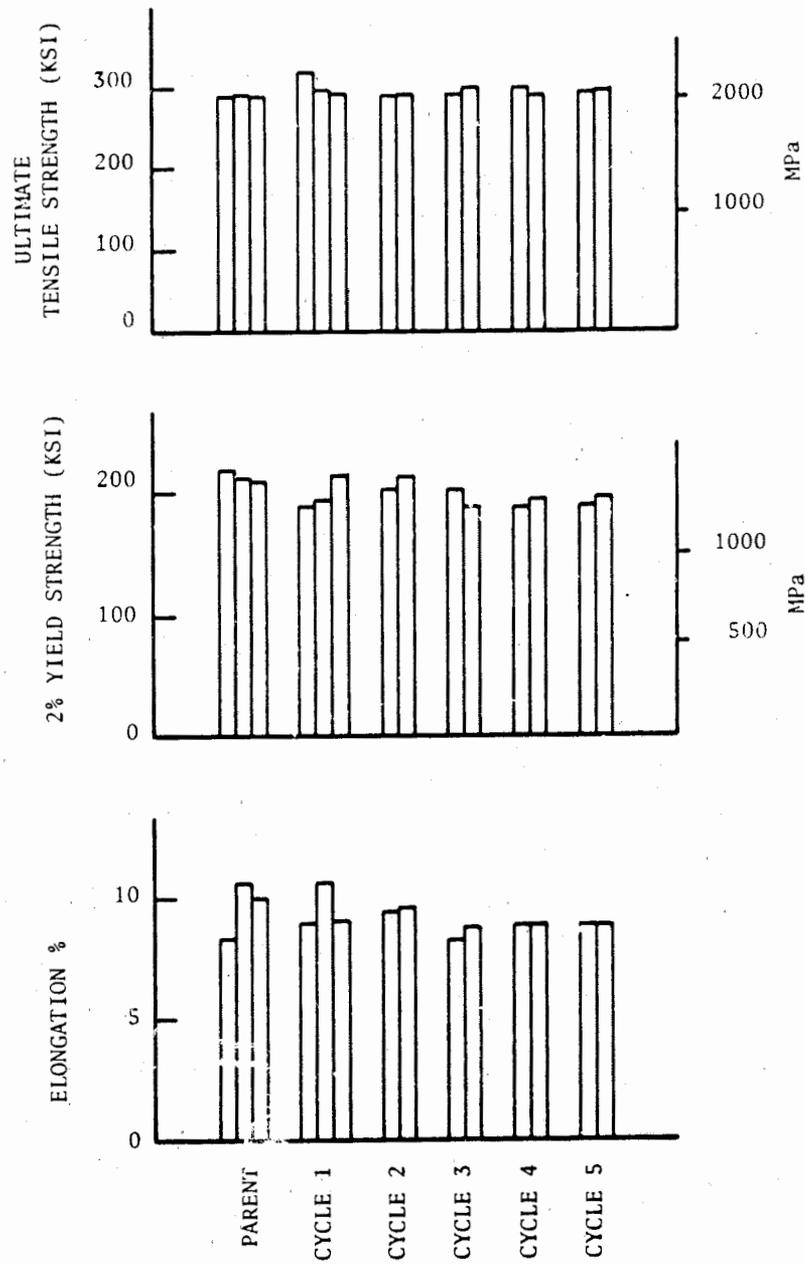
Figure 15 - Tensile Properties Results
