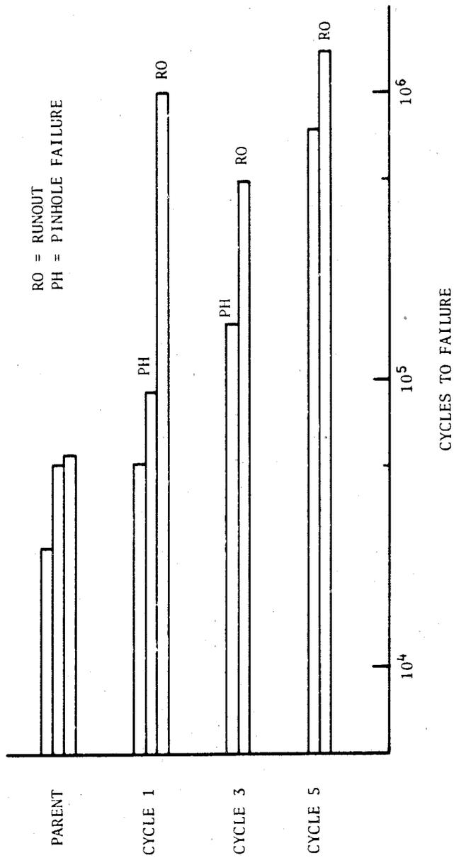
Figure 16 - Fatigue test data, 170 ksi test stress and +0.1 R ratio
