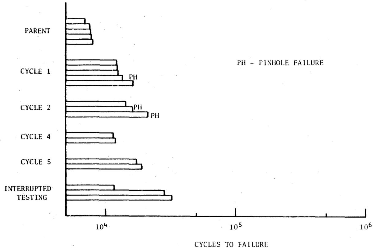
Figure 19 - Fatigue test data, 200 ksi test stress and -0.3 R ratio
