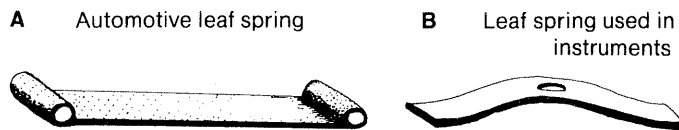
Fig. 13. A, Leaf spring stressed in one direction only; B, leaf spring stressed in two directions.
