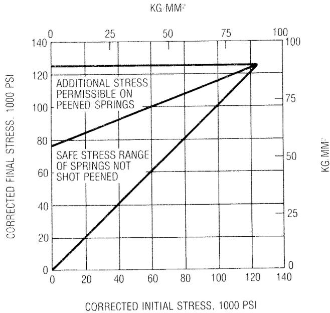
Fig. 4 SAFE STRESS RANGES FOR COIL SPRINGS (.207 DIAMETER STEEL)
