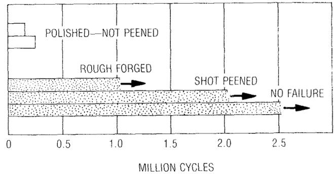
Fig. 9. FATIGUE DURABILITY OF FORK TYPE CONNECTING RODS
