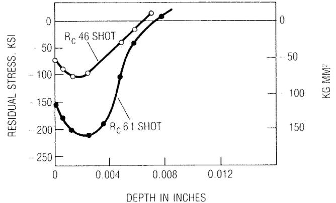
Fig. 3. PEENING 1045 STEEL AT Rc62 WITH 330 SHOT
