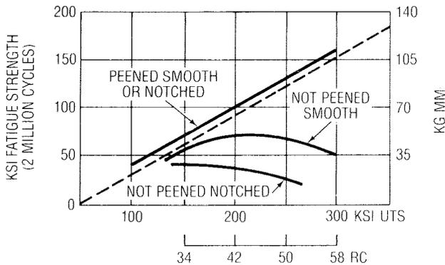
Fig. 2. COMPARISON OF PEENED AND UNEPEENED FATIGUE LIMITS FOR SMOOTH AND NOTCHED SPECIMENS AS A FUNCTION OF ULTIMATE TENSILE STRENGTH OF STEEL.
