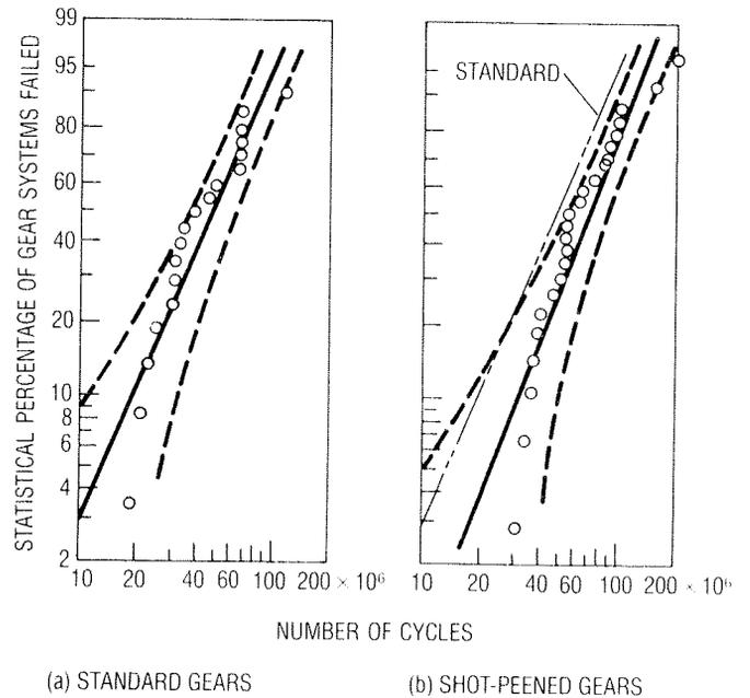
Fig. 7. COMPARISON OF SURFACE (PITTING) FATIGUE LIVES OF STANDARD GROUND AND SHOT-PEENED CARBURIZED AND HARDENED CVM AISI 9310 STEEL SPUR GEARS. SPEED, 10,000 RPM; LUBRICANT, SYNTHETIC PARAFFINIC OIL; GEAR TEMPERATURE, 350 K (170 F); MAXIMUM HERTZ STRESS,  $1.7 \times 10^9$  N/m<sup>2</sup> (248,000 PSI).
