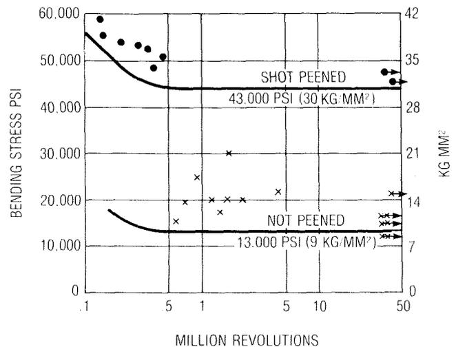
Fig. 10. FATIGUE TESTS ON REAR AXLE SHAFTS
