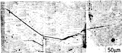
a) Baseline condition \sigma_a = 300 \text{ MPa} N_F = 3.1 \times 10^4
