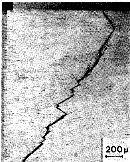
Fig. 4. Crack path in 8090 tested in plain fatigue.
