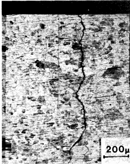
Fig. 5. Crack path in 7010 tested in plain fatigue.
