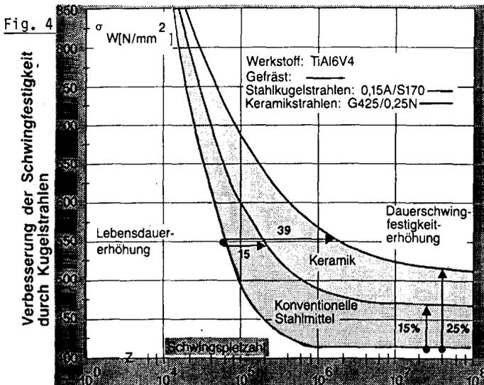
The Wöhler diagrams in Fig. 4 show the mean-value curves (50% probability of survival) obtained using a modified Weibull method. Results for smooth specimens are shown in Figs. 4 and 5. Using conventional peening media such as glass, steel or old ceramic, the fatigue limit can be improved from 410 to 470  $N/mm^2$ , which is equivalent to an improvement of 15%. Using new ceramic or zirshot, however,
