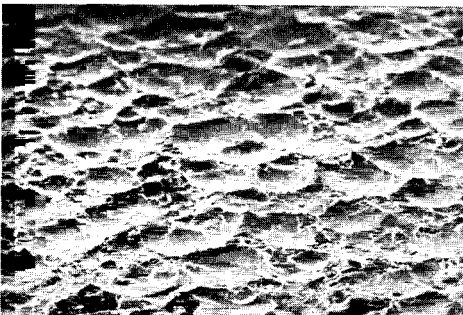
Fig. 5: 54:1 Peening media : MGL 0,42 - 0,84 mm coverage : A* = 12 x 98%
