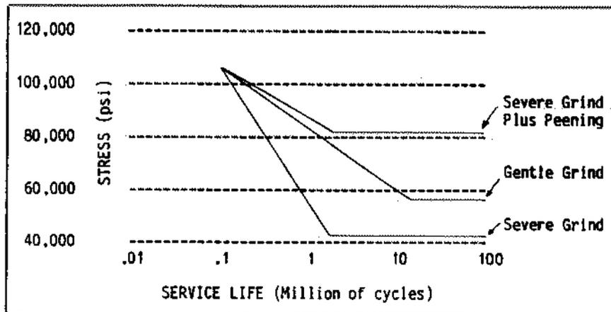
Fig. 1. Representative increase in resistance to cyclical loading produced by peening.
