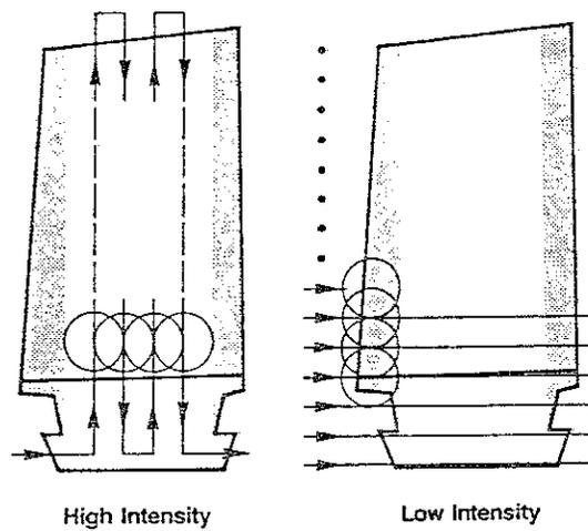
Fig. 60: Shot peening of thin blades (schematic).
