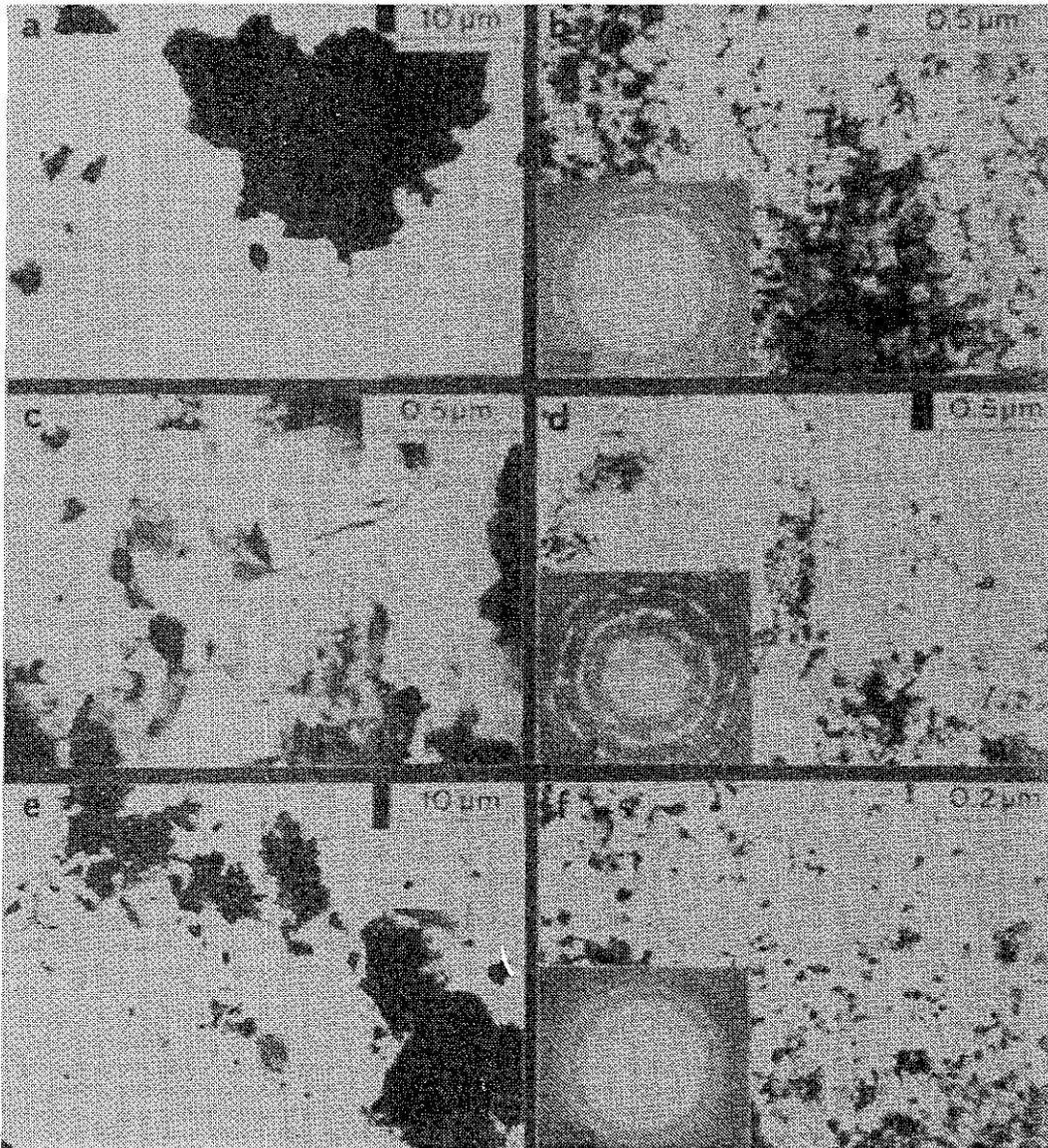
Fig. 16: Transmission electron microscopy of erosion debris and cold rolled material.
