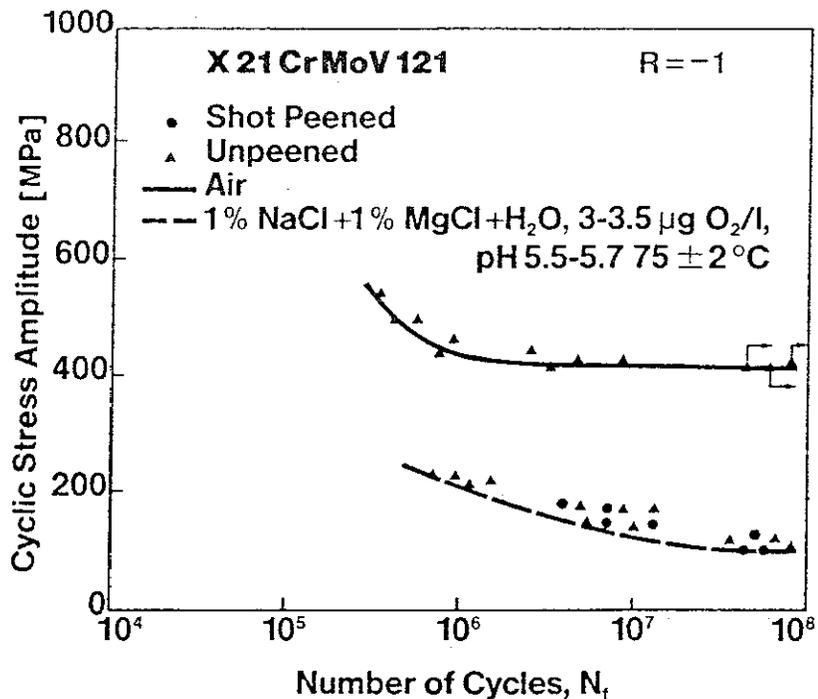
Fig. 43: SN-curves for shot peened and unpeened specimens tested in air and in a corrosive environment.
