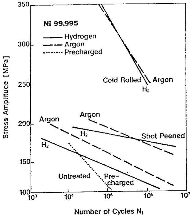
Fig. 45: SN-curves for different treated specimens, tested in different environments.
