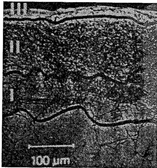
Fig. 6: Zones of different deformation after shot peening of A286, visible after heat treatment: 24h, 820 °C.
