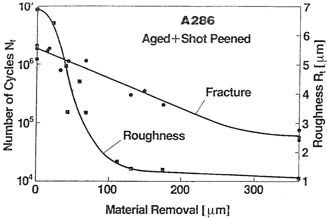
Fig. 31: Influence of surface material removal on the roughness and number of cycles to failure of shot peened A286 ( $\sigma_a = 550$  MPa,  $f = 25$  Hz, air,  $R = -1$ )
