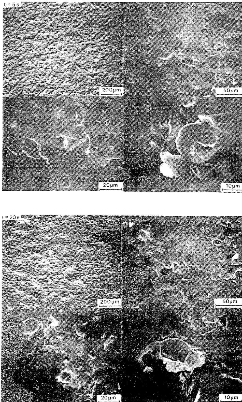
Fig. 12: Surface appearance after shot peening for different times.
