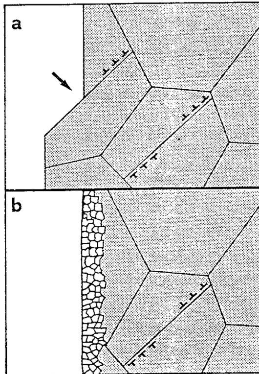
Fig. 47 a: Formation of slip bands in an untreated surface. b: Cross-section of a shot peened and recrystallised surface layer (schematic).
