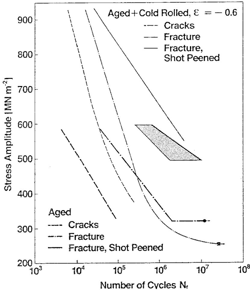
Fig. 23: Influence of cold rolling and shot peening on the fatigue strength of A286.
