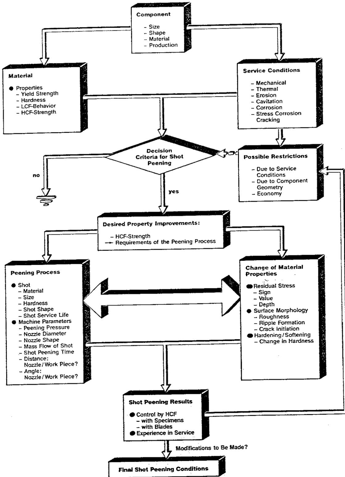
Fig. 49: Procedure to fix the peening conditions (schematic).
