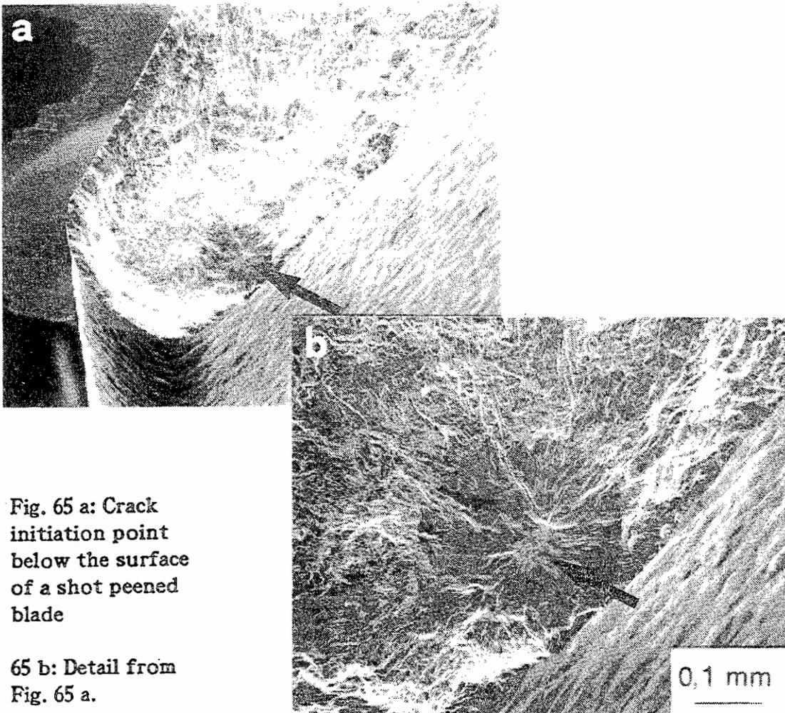
Fig. 65 a: Crack initiation point below the surface of a shot peened blade
