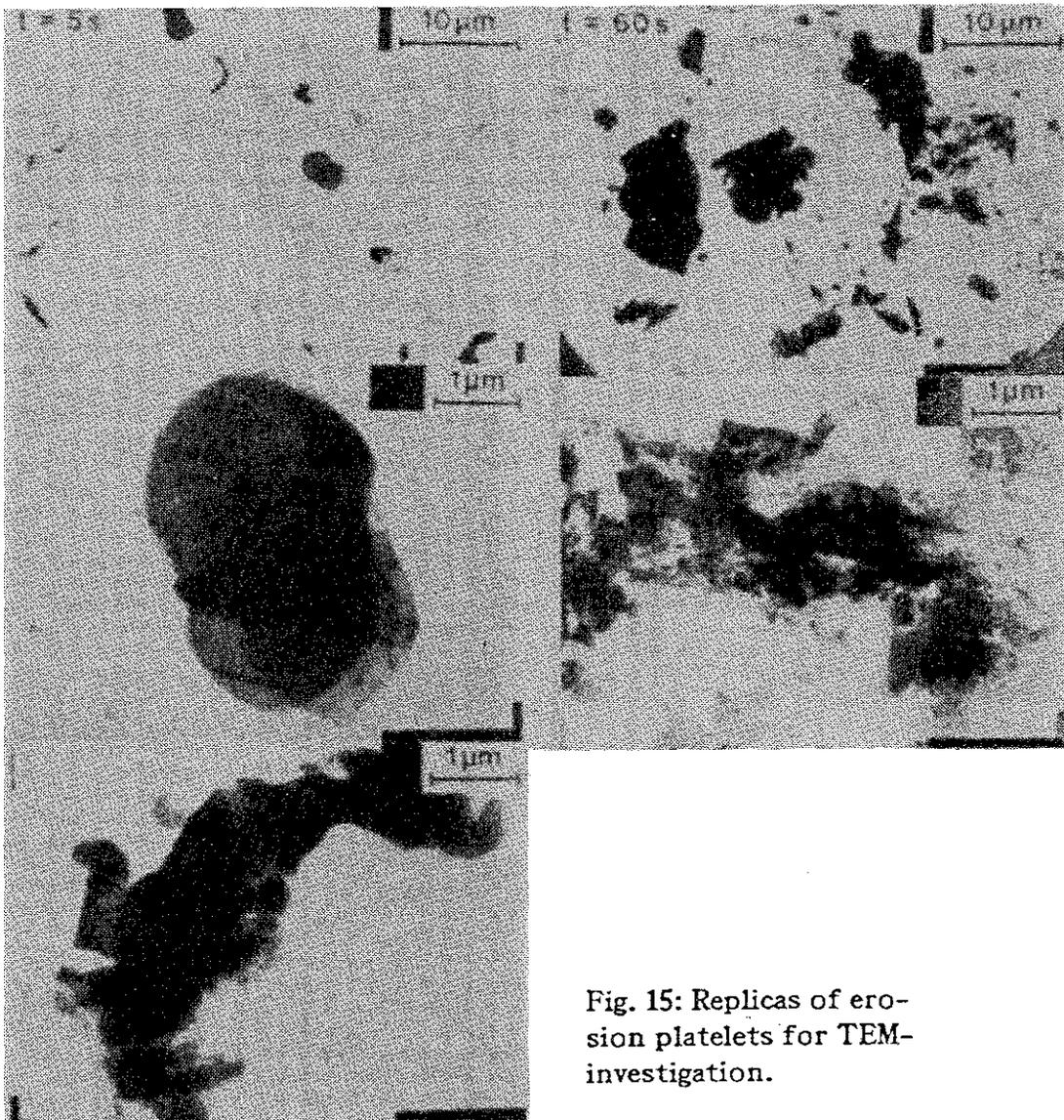
Fig. 15: Replicas of erosion platelets for TEM-investigation.
