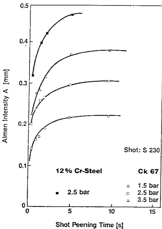
Fig. 55: Almen intensity as a function of shot peening time for constant peening
