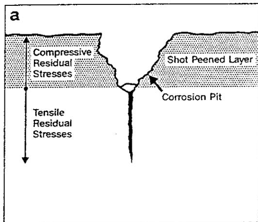
Fig. 44 a: Stress corrosion failure nucleating from an etch pit in a shot peened surface (schematic).
