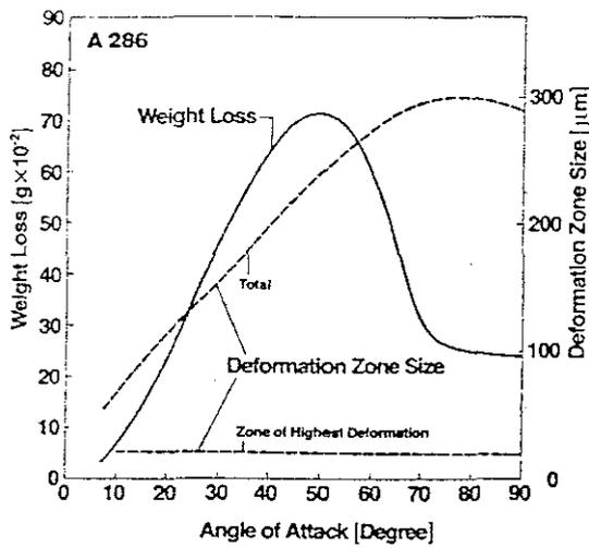
Fig. 10: Deformation depth and weight loss as a function of angle of attack.
