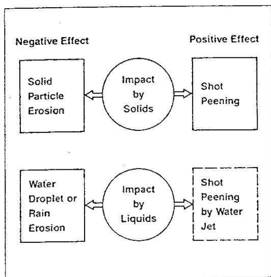
Fig. 34: Positive and negative effects of solid and liquid impact.
