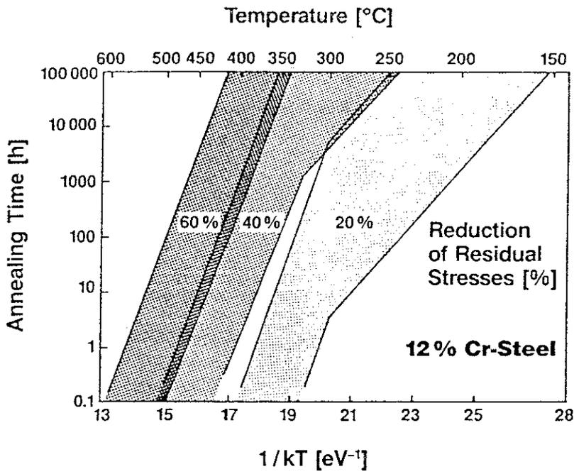
Fig. 48: Prediction of the residual stress relief as a function of annealing time and temperature.
