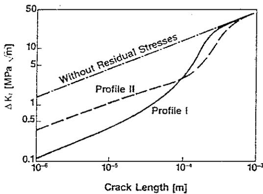
Fig. 38: Dependence of calculated ranges of stress intensities  $\Delta K$  on simulated residual stress profiles.
