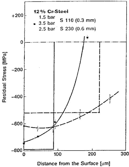
Fig. 57: Comparison of measured residual stress profile and calculated rectangular stress profiles.
