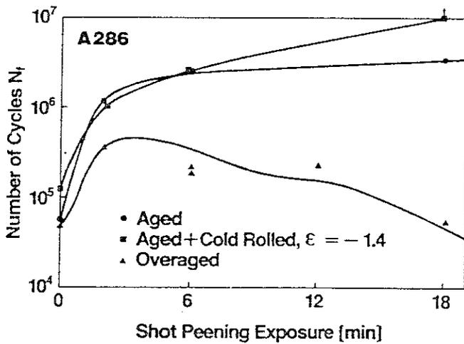
Fig. 27: Influence of shot peening time on the fatigue life of A286
