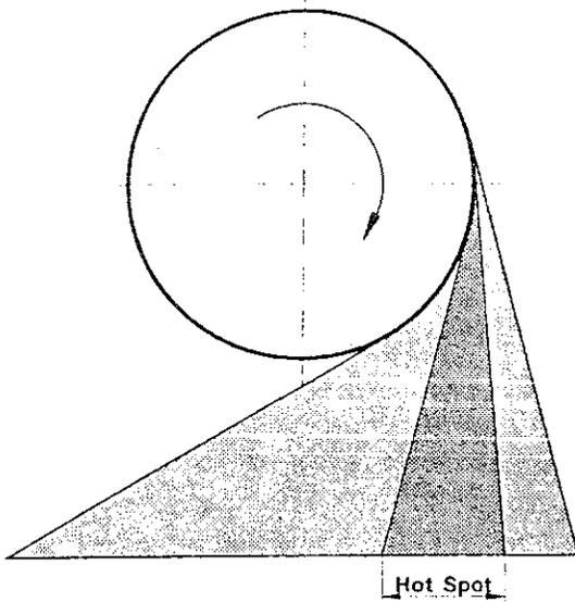
Fig. 51: Peening patterns of a centrifugal wheel machine (schematic).
