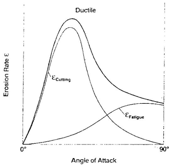
Fig. 14: Solid particle erosion as a function of the impact angle.
