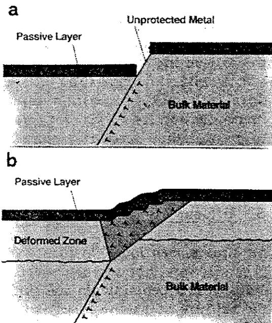
Fig. 42: Influence of shot peening on corrosion fatigue crack initiation (schematic)
