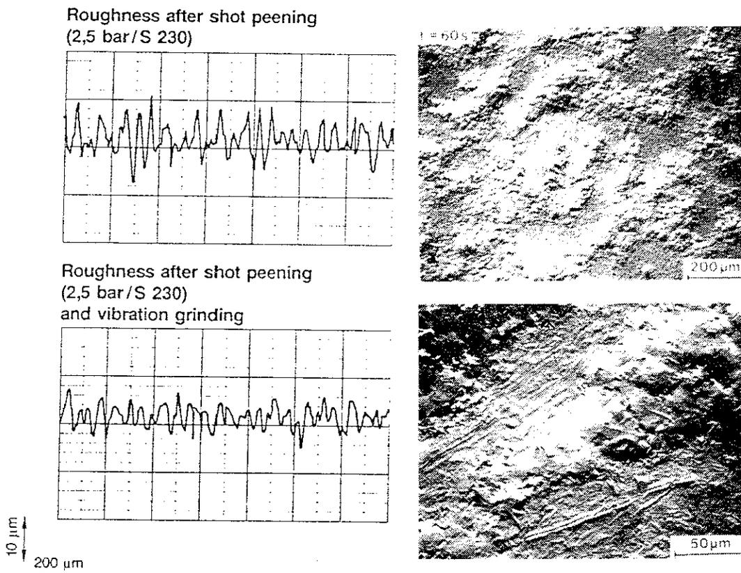
Fig. 30: Influence of vibration grinding on the roughness of a shot peened surface.
