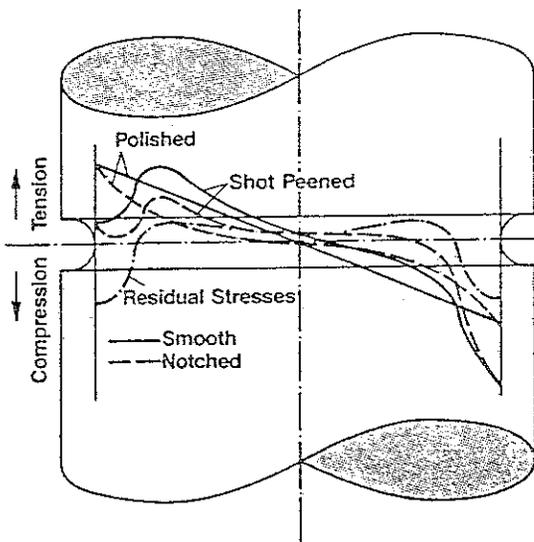
Fig. 59: Superimposition of applied stresses (bending) and residual stresses (shot peening treatment) for a notched and an unnotched specimen (schematic).
