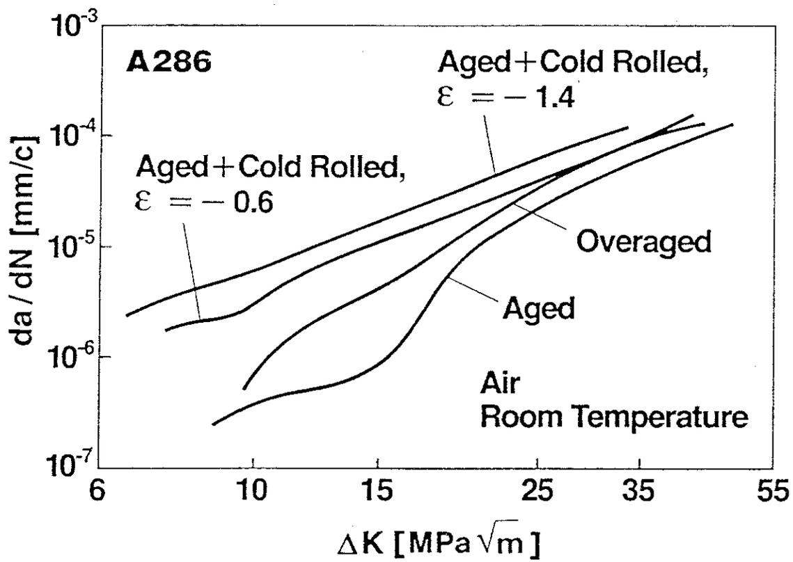
Fig. 25: Fatigue crack propagation rate for different conditions of A286.
