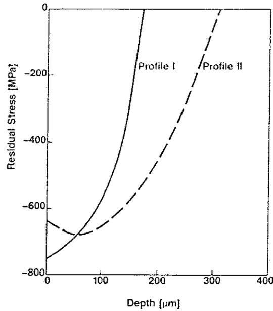
Fig. 37: Different simulated residual stress profiles in the surface layer.
