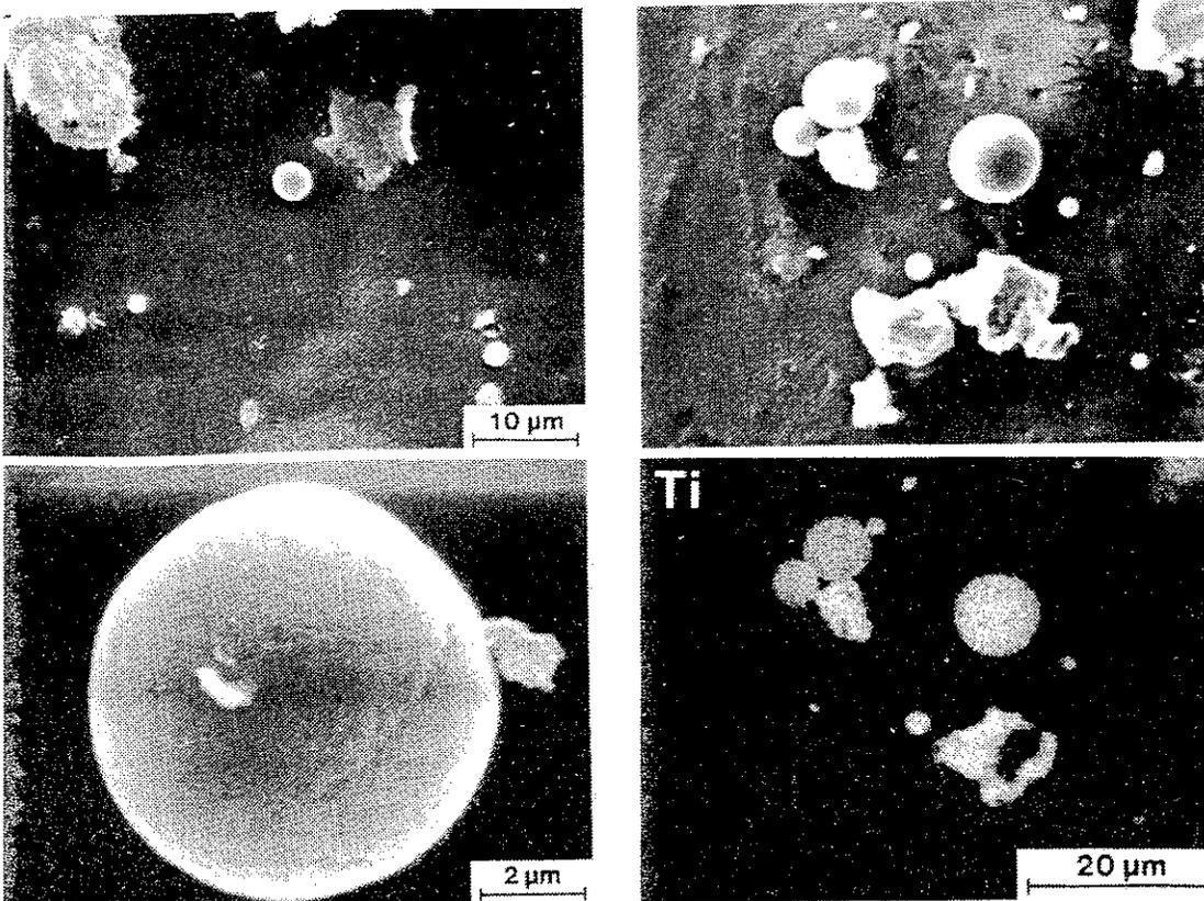
Fig. 19: Ti droplets and platelets after shot peening
