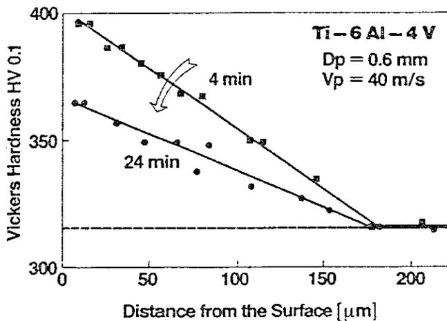
Fig. 28: Microhardness profile in the surface layer after shot peening for different peening times /17/.
