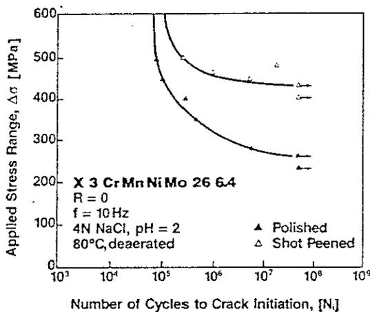
Fig. 41: SN-curves for polished and shot peened specimens tested in corrosive environment
