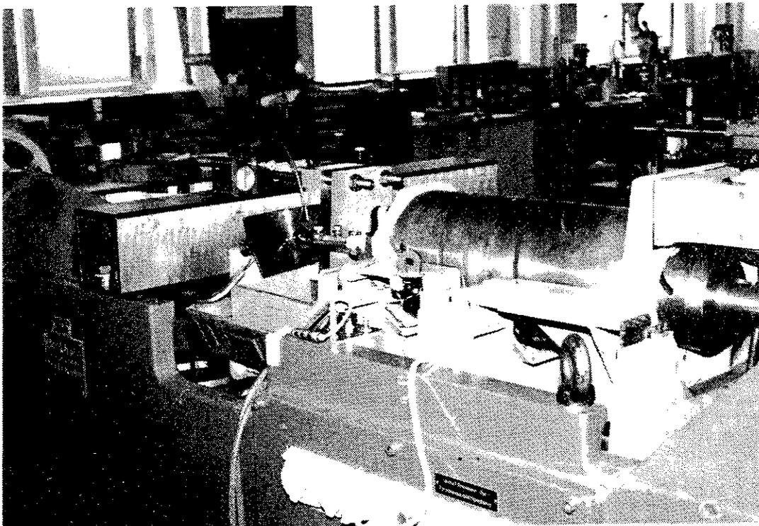
Fig. 63: Test arrangement for fatigue testing of compressor blades.
