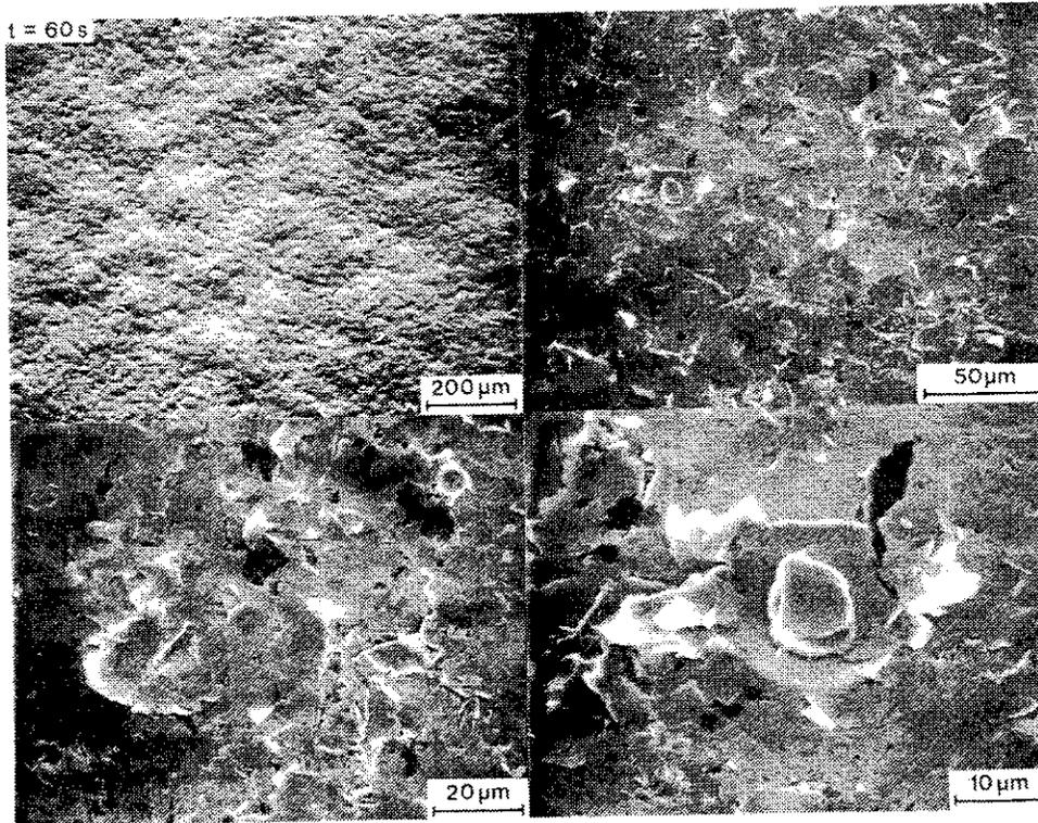
Fig. 12: Surface appearance after shot peening for different times.
