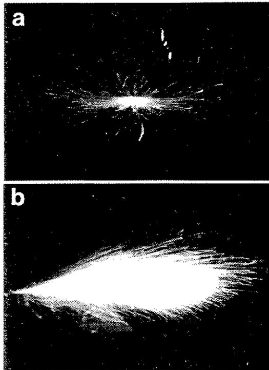
Fig. 18: Shot peening of titanium at a) 90° and b) at 30° impact angles (Exposure time 2 min.)
