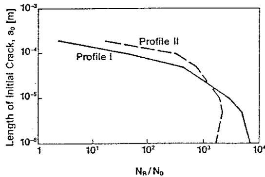
Fig. 39: Increase in fatigue life as a function of starter crack length and the residual stress profile.
