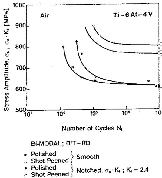
Fig. 58: SN-curves, influence of shot peening on the fatigue limit of notched and unnotched specimens (Air, R = -1, RT).
