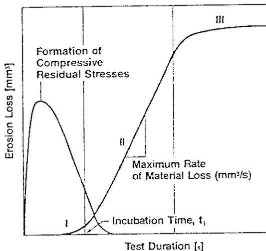
Fig. 35: Water droplet erosion and formation of compressive residual stresses.
