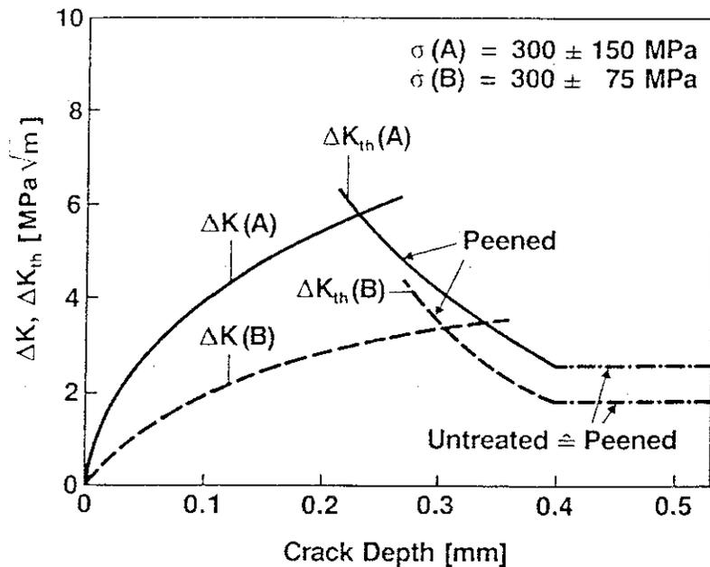
Fig. 40: Stress intensity ( $\Delta K$ ) and threshold stress intensity values ( $\Delta K_{th}$ ) for shot-peened and untreated samples as a function of crack depth.
