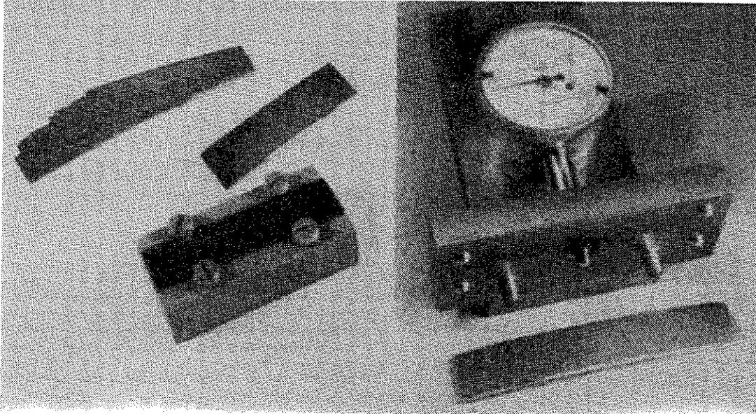
Fig. 54: a) Almen test strips and fixture.
