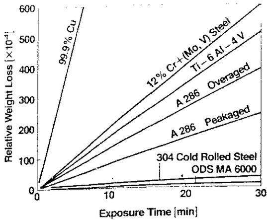
Fig. 17: Erosion weight loss for various turbine blade materials.
