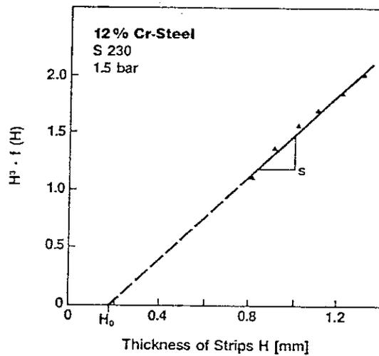
Fig. 56: Plot of deflection data against plate thickness. The  $H_0$ -value and the slope  $s$  can be used for calculating a rectangular or a parabolic stress profile
