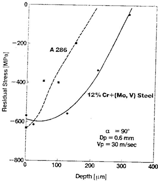
Fig. 5: Residual stress distribution of A286 and 12% Cr-steel after shot peening (S230).
