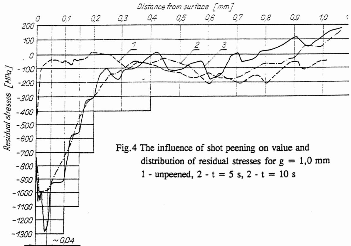
Fig.4 The influence of shot peening on value and distribution of residual stresses for  $g = 1,0$  mm
