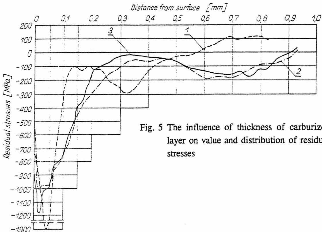
Fig. 5 The influence of thickness of carburized layer on value and distribution of residual stresses
