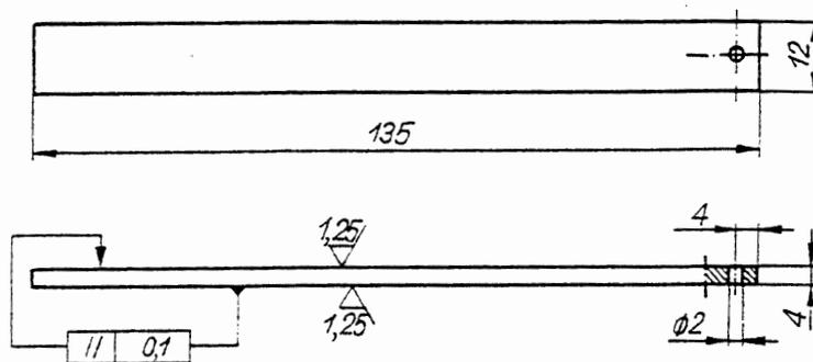
Fig. 2 Specimen for measurement of value and distribution of residual stresses.
