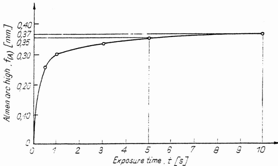
Fig. 1 Shot peening saturation curve.
