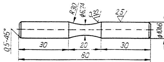
Fig. 6 Specimen for testing fatigue strength
