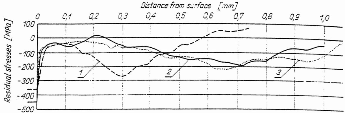
Fig. 3 The influence of thickness of carburized layer on value and distribution of residual stresses.
