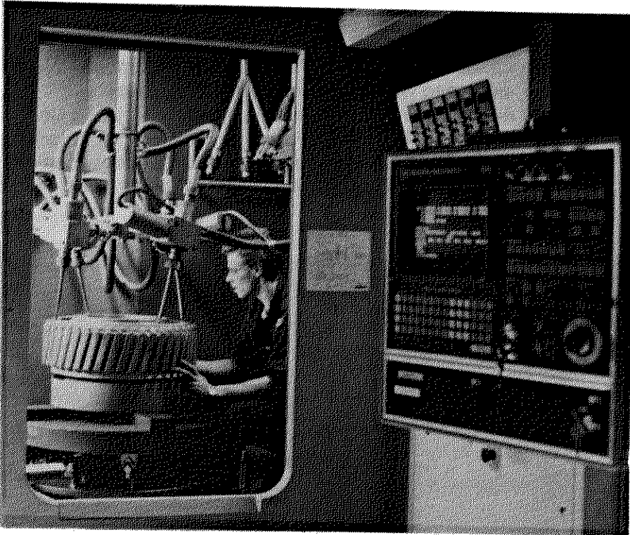
Efficient slope slot peening, with four simultaneously moving internal rotation peening heads used on a NORSK JETMOTOR Multi-purpose Shot Peening Plant (Series 5) in Norway.
