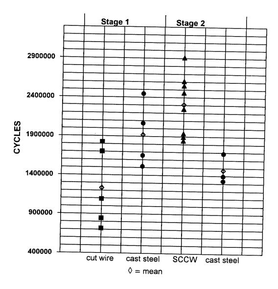
Figure 3 - Fatigue Test Results
