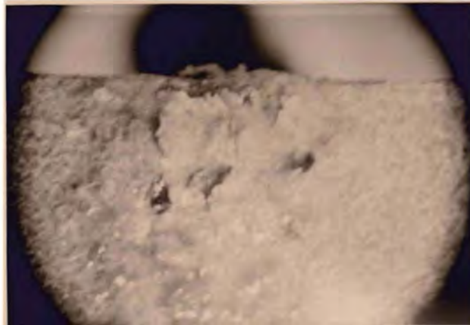
Fig 6: Sever pitting and cracking after 211hr exposure, when shot peened at 8A intensity (30X)
