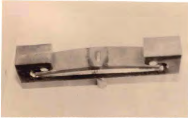
Fig 4: The attack in HAZ of the un-peened specimens
