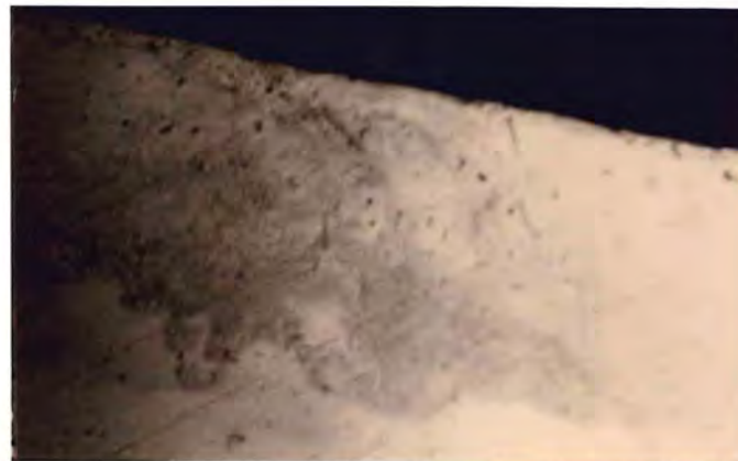
Fig 3: Effect of Shot Peening at an intensity of 10A (100X) (Dept of compressive layer=0.53mm).
