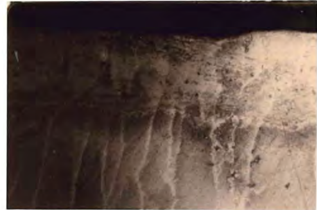
Fig 2: Effect of Shot peening at an intensity of 8A (100X) (Depth of Compressive layer=0.35mm),
