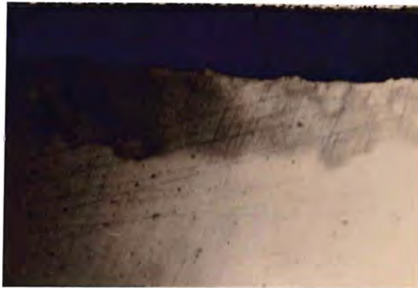
Fig 1: Effect of shot peening at an intensity of 6A (100X) (Depth of compressive layer-0.24mm)
