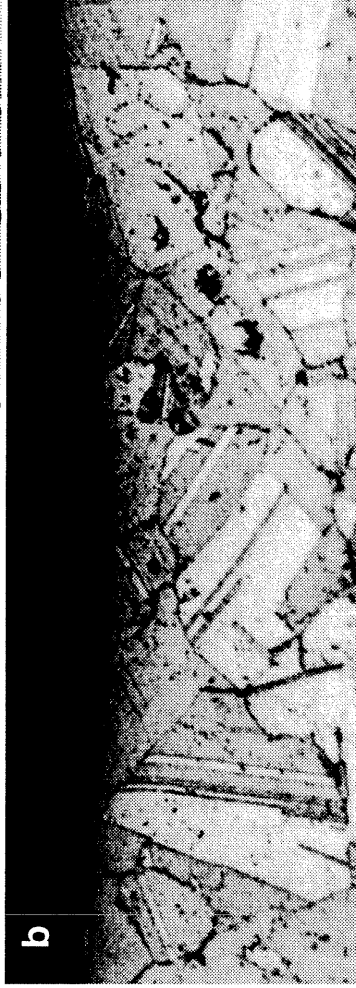
b) 3-017, ccw1404, R88-04 || 87.5 m/s in 46.7 m/s out 90° incidence
