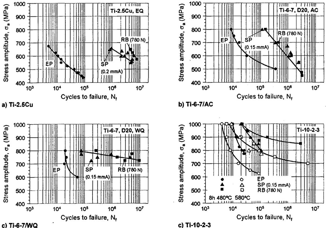
**Fig. 8: S-N curves of the various titanium alloys, Effect of shot peening or roller-burnishing**
