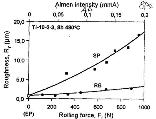
Fig. 4: Surface roughness after mechanical surface treatment in Ti-10-2-3
