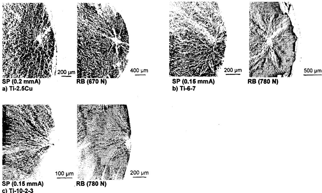
Fig. 9: HCF crack nucleation sites after mechanical surface treatments
