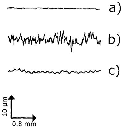
Fig. 3: Surface profiles after various surface treatments in Ti-10-2-3, 8h 480°C
