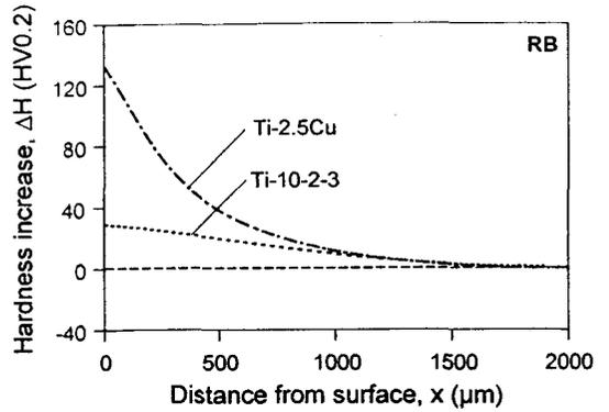
Fig. 5: Hardness profiles after shot peening or roller-burnishing
