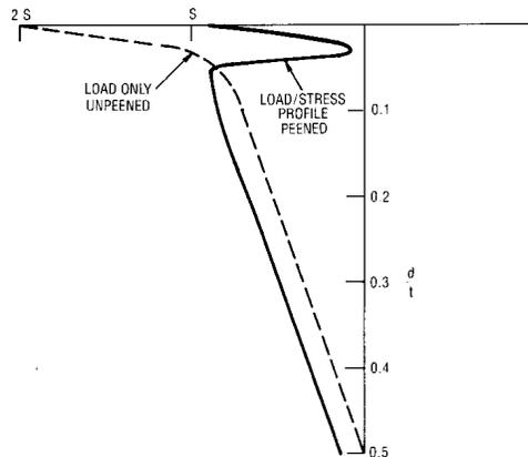
Fig. 6 Load/Stress Distribution of Shot Peened Notched Beam under Bending Load
