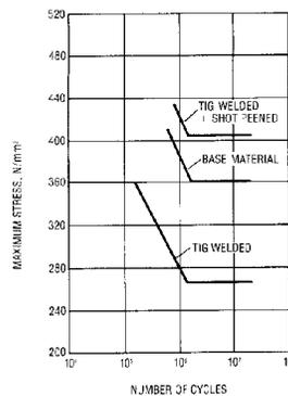
Figure 16 Effect of Shot Peening on Welded STE690 Material
