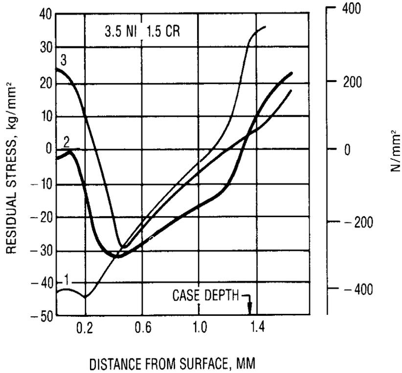
Fig. 18 The Effect of Decarburization on the Residual Stresses Developed in Carburized and Hardened Plates.
