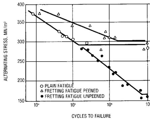
Fig. 20 Rotating-Bending Fatigue Curves for Untreated and Shot-Peened Specimens of Annealed Austenitic Stainless Steel En 58A With and Without Fretting
