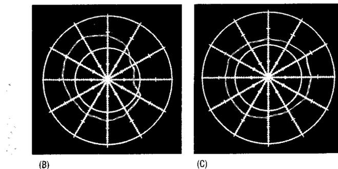
FIG. 46 Contour Correction of Ring Gear
