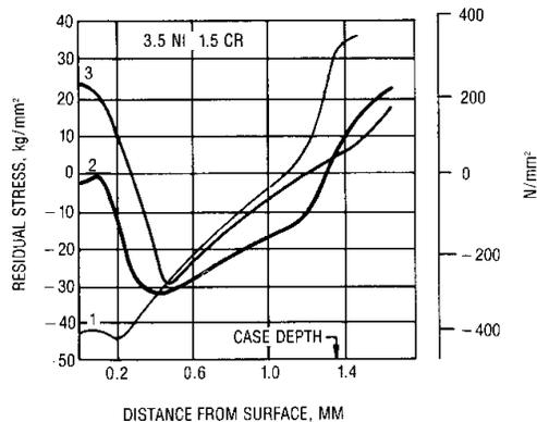
Fig. 17 Effect of Shot Peening on Decarburization
