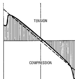
Fig. 4 Superposition of Applied and Residual Stress
