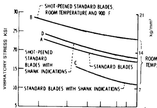
Fig. 26 Suppression of Fatigue Damage of Inconel 713c Turbine Blades by Shot Peening
