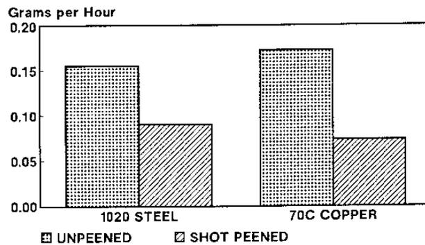
Fig. 19 Rate of Material Loss by Cavitation
