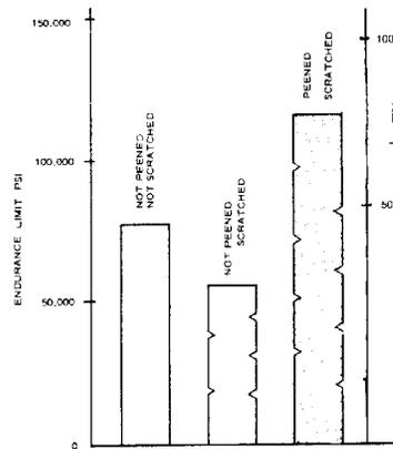
Fig. 28 Effect of Peening and Scratches on Endurance Limit of 4340 Steel at Rc51
