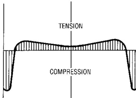
Fig. 3 Typical Residual Stress Distribution After Peening
