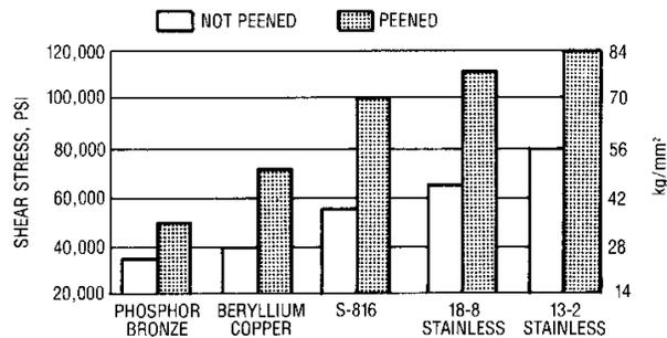
Fig. 37 Safe Stress Ranges for Coil Springs of Various Alloys
