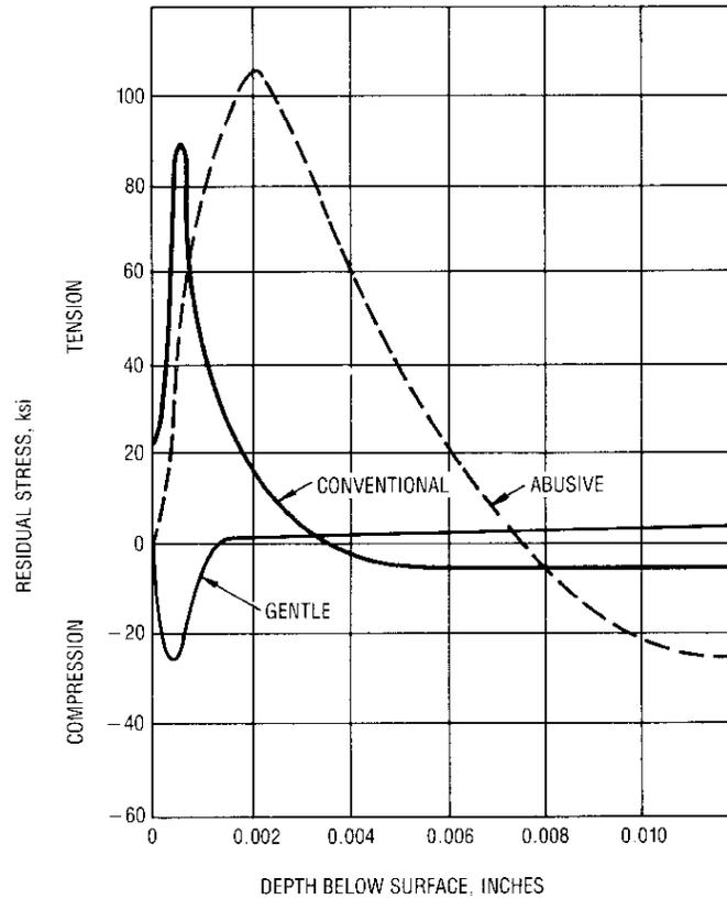
Fig. 8 Residual Stress in 4340 Steel (Hrc50) After Surface Grinding
