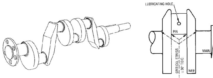
Fig. 31 Crankshaft and Detail
