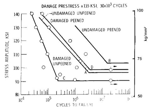
Fig. 27 Shot Peening as a Means of Overcoming Prior Fatigue Damage with 4340 Steel Tested in Rotating Bending
