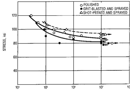
Fig. 13 The Influence of Hard Anodizing and Shot Peening on the Failure Strength of Duralumin (LI)
