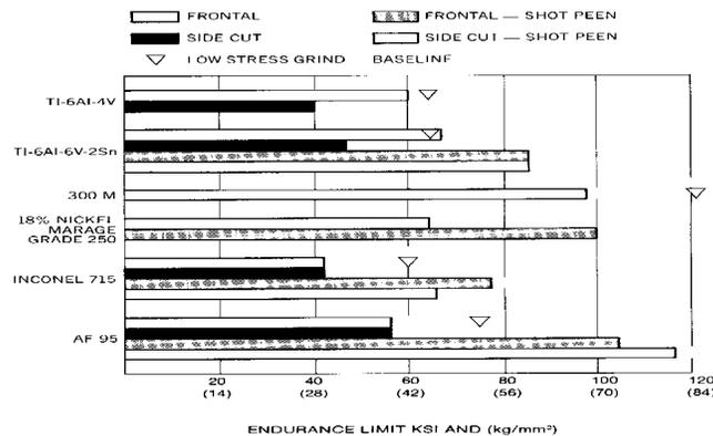
Fig. 10 Summary of High-Cycle Fatigue Response for ECM
