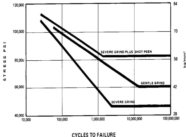
Fig. 7 Reversed Bending Fatigue of Flat Bars of Rockwell Hardness C45
