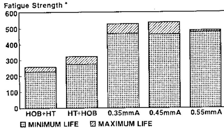
Figure 42 The Effect of Processing Variables on the Bending Fatigue Strength of Austenitic-bainitic (K9805) Gear-teeth: Measured after 10 Loading Cycles.
