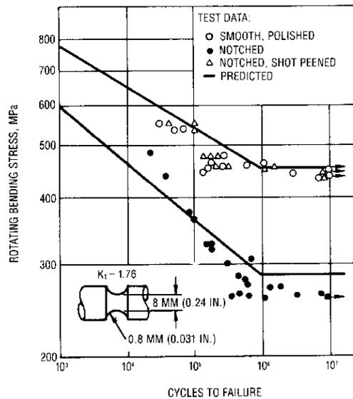
Fig. 36 Fatigue Tests on Notched Shafts
