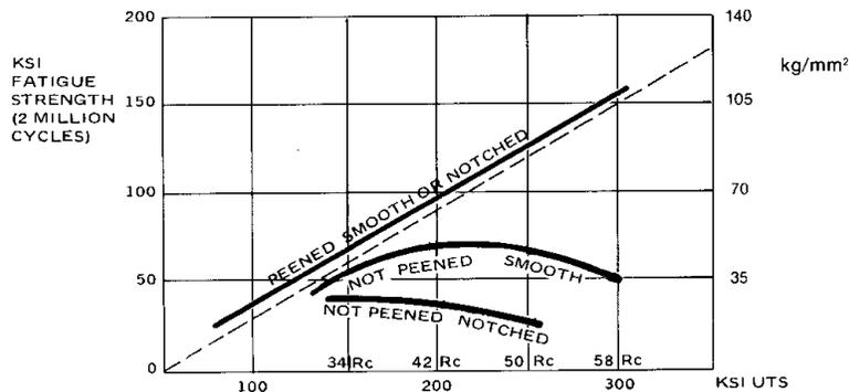
Fig. 39 Comparison of Peened and Unpeened Fatigue Limits for Smooth and Notched Specimens as a Function of Ultimate Tensile Strength of Steel
