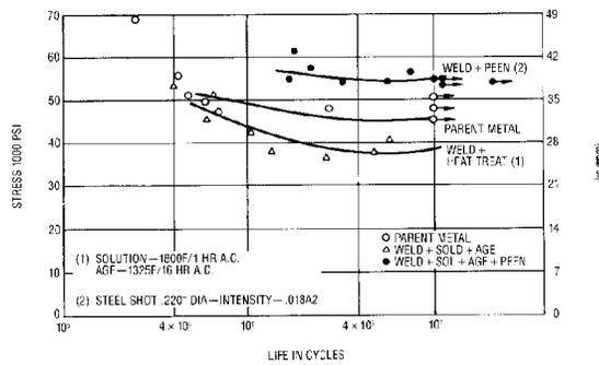
FIG. 15 Effect of Shot Peening on Welded A-286 Fatigue Strength
