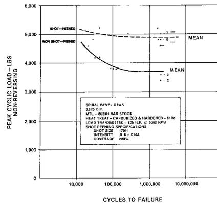
Fig. 32 Increase in Fatigue Resistance of Spiral Bevel Gear
