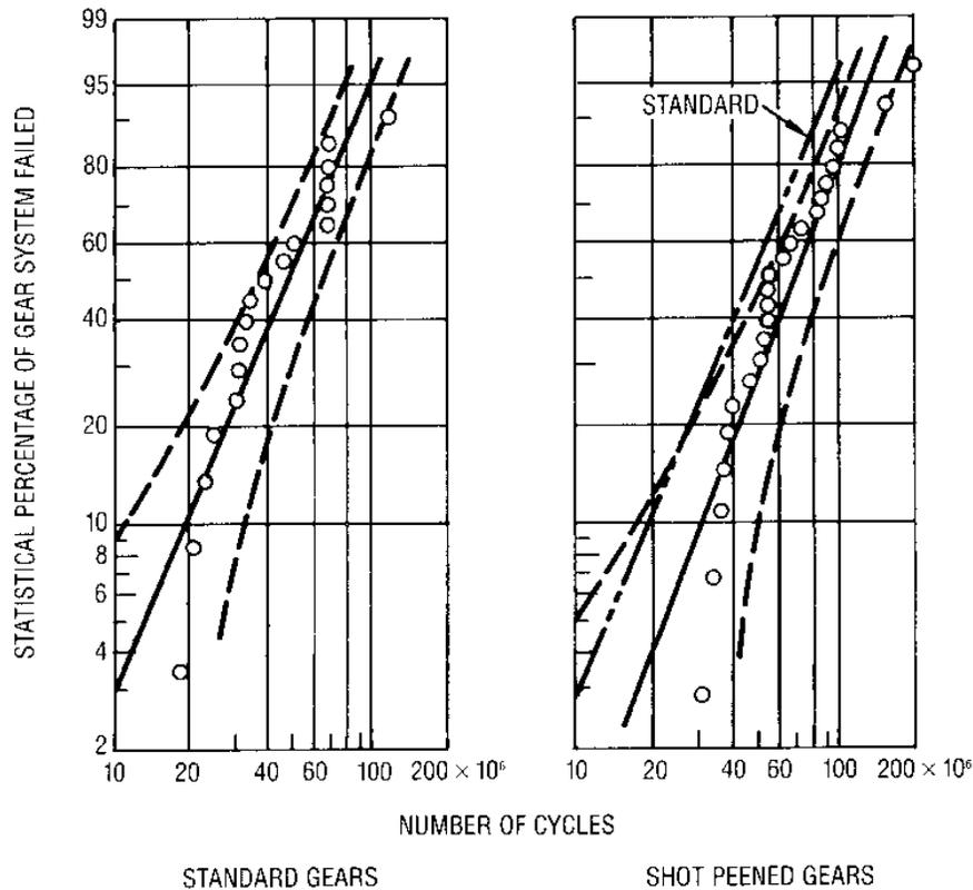
Fig. 23 Comparison of Surface (Pitting) Fatigue Lives of Standard Ground and Shot-Peened Carburized and Hardened CVM AISI9310 Steel Spur Gears, Speed, 10,000 RPM; Lubricant, Synthetic Paraffinic Oil; Gear Temp. 350K (170 f) Maximum Hertz Stress,  $1.7 \times 10^8$  N/m (248,000 psi)
