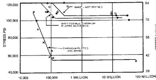
Fig. 12 Cycles to Failure 4340 Steel, 52-53Rc Rotating-Beam Fatigue
