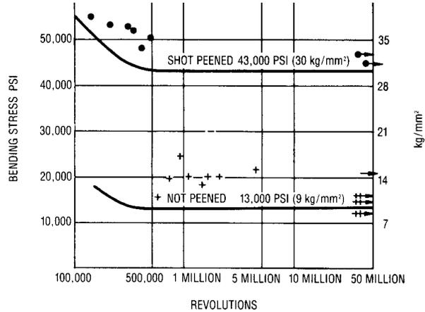
Fig. 35 Fatigue Tests on Rear-axle Shafts
