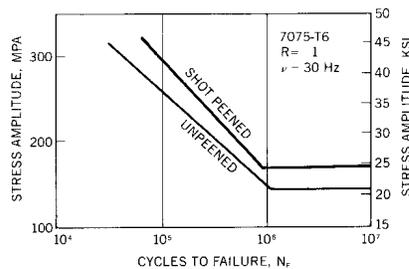
Fig. 40 Results of Reversed Bending Fatigue Tests on Unpeened and Peened Specimens of 7075-T6 Aluminum Alloy
