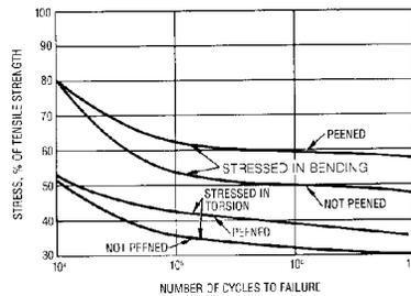
Fig. 38 Comparison of Fatigue Curves Bending Vs. Torsion Loading
