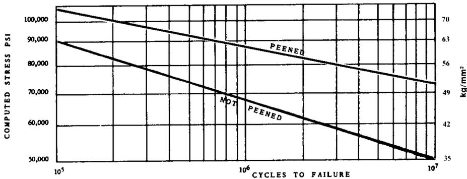
Fig. 34 Fatigue of Carburized Gears
