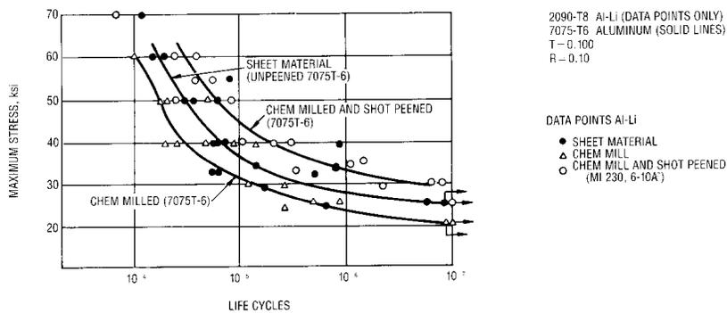
Fig. 41 Comparison of 7075-T6 Vs. Al-Li Fatigue Results
