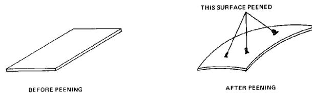
Fig. 44 Compound Curvature Result of Tri-axial Forces Induced by Shot Peening
