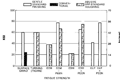
Fig. 9 Summary of High-Cycle Fatigue Behavior on Inconel 718, Solution-Treated and Aged (Rc44)
