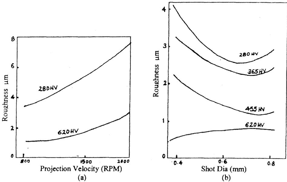
Fig.2. Effect of (a) Projection Velocity 9b) Shot dia, on the surface finish
