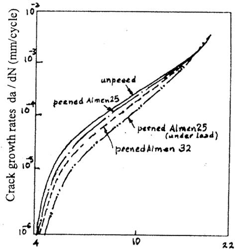
Fig.6 b. Crack growth rate behaviour of specimen for Life prediction
