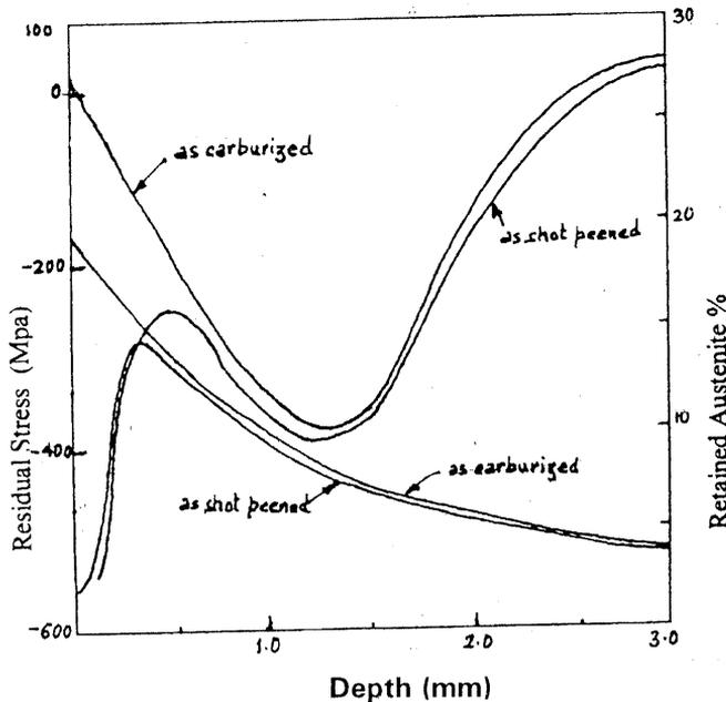
Fig.4 Distribution of residual stresses and retained austenite in as carburized and shot peened-carburized steel.
