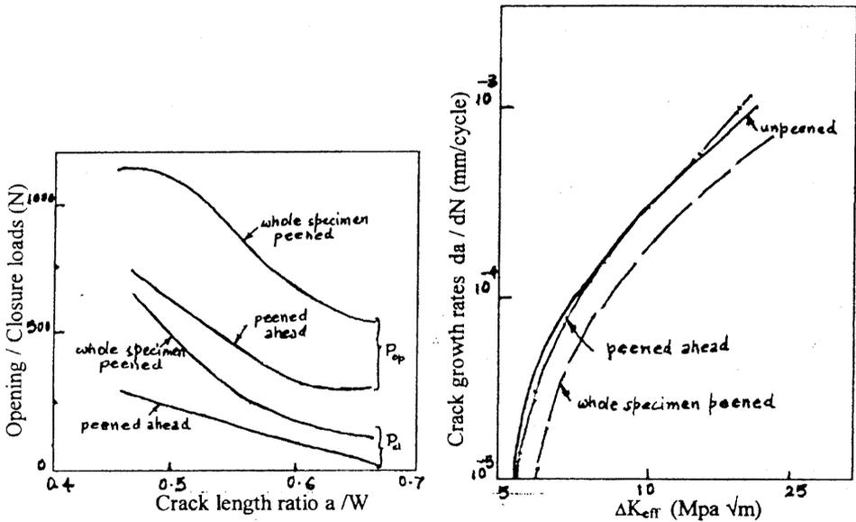
Fig.5a. Crack opening / closure levels at different peening different locations
