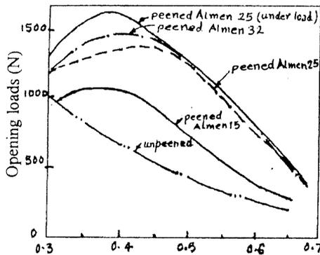
Fig.6 a. Crack opening levels at various peening conditions different peening conditions
