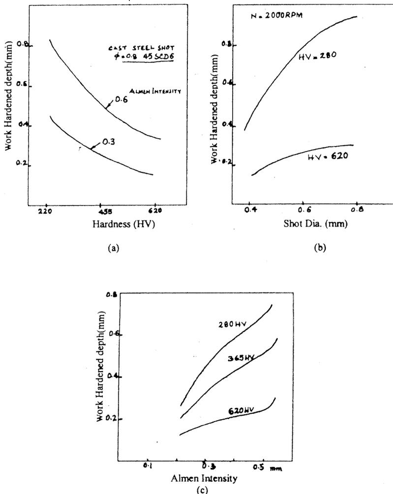
Fig.1. Effect of Material Hardness, Shot Dia, Almen Intensity on Work Hardening Depth.
