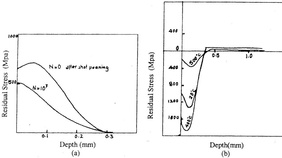
Fig.3. Stress relaxation after shot peening due to
