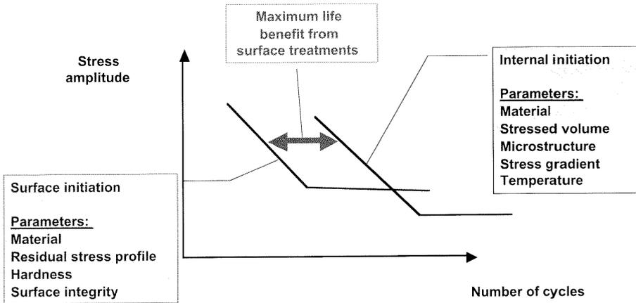
Figure 3: Surface crack initiation vs. internal crack initiation
