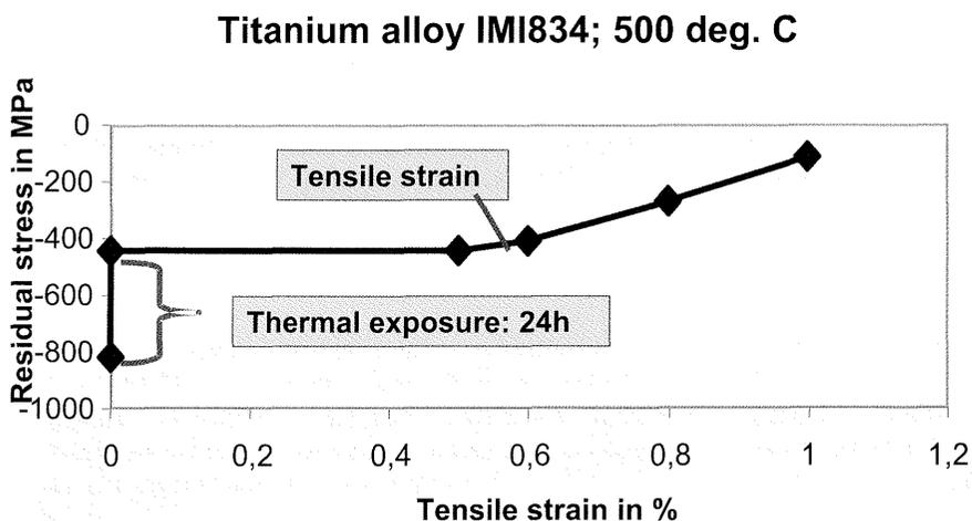
**Figure 11:** Modeling of residual stress shake-down caused by thermal exposure and subsequent tensile strain at 500 deg. C
