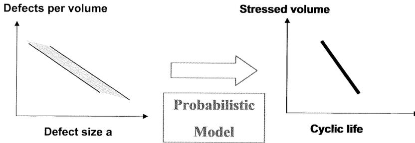
Figure 13: Volume-dependent cyclic life due to the statistical size effect
