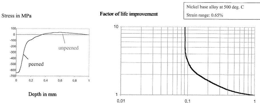
Figure 14: Decreasing life benefit with increasing defect size Residual stress depth profile (left) Fracture mechanics calculation for a semi-circular surface defect (right)
