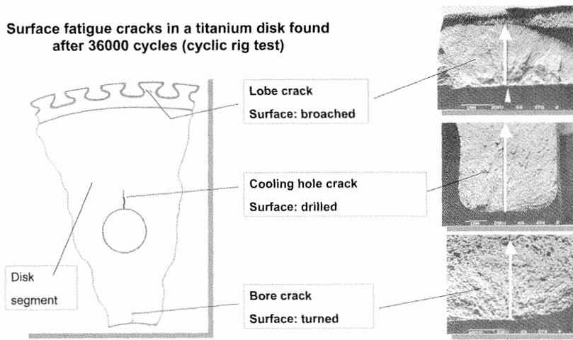
**Figure 1:** Example of surface crack initiation at various locations of a compressor disk
