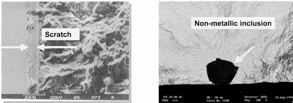
**Figure 6:** Examples of crack-like surface defects found at the origin of fatigue cracks Scratch produced by handling - Non-metallic inclusion (nickel base alloy)
