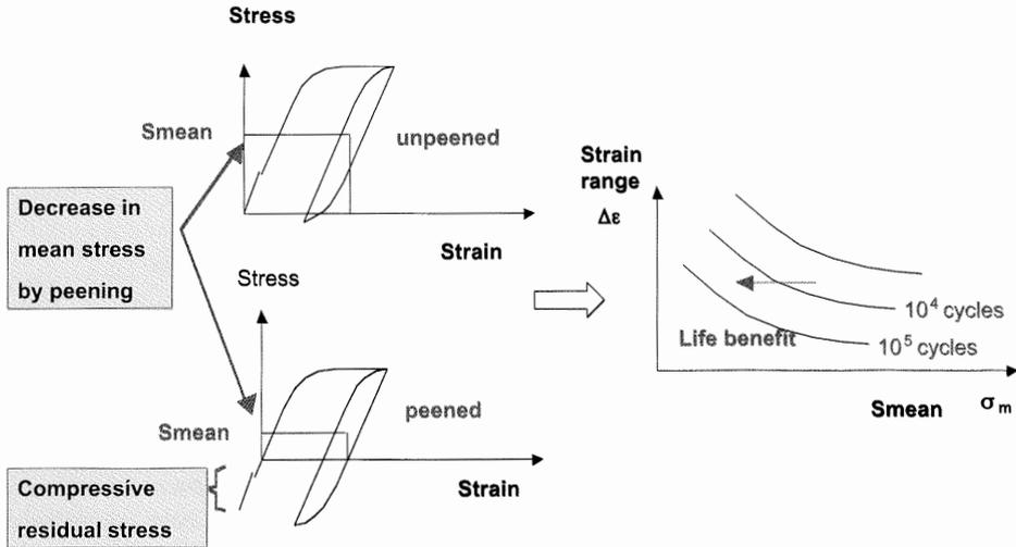
**Figure 5:** Model to predict the benefit of compressive residual stresses on fatigue life caused by a reduction of the mean stress  $S_{mean}$
