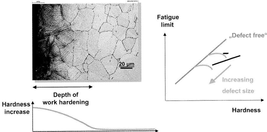
Figure 4: Fatigue strength increases with hardness; defects disturb this relationship
