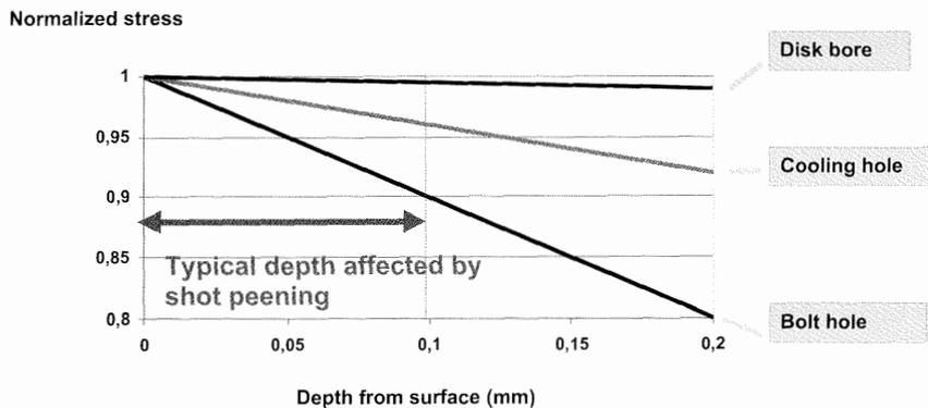
**Figure 2:** Stress gradient below the surface for various disk features (bore, cooling and bolt hole)
