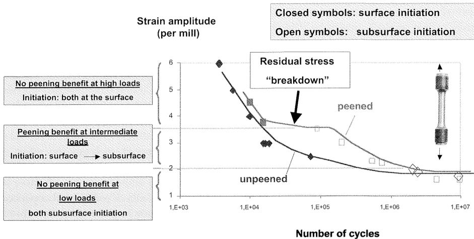
Figure 12: Effect of peening on LCF life (nickel base alloy)
