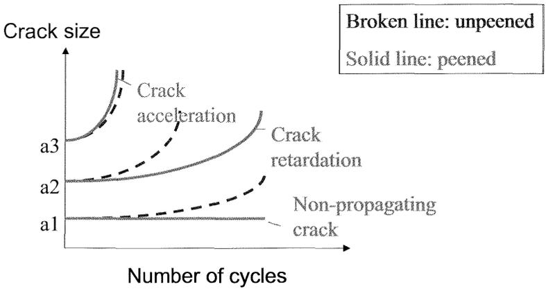
Figure 7: Effect of shot peening on the propagation behavior of surface cracks
