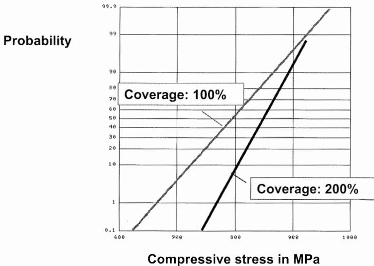
**Figure 10:** Influence of coverage on mean values and scatter of residual stresses
