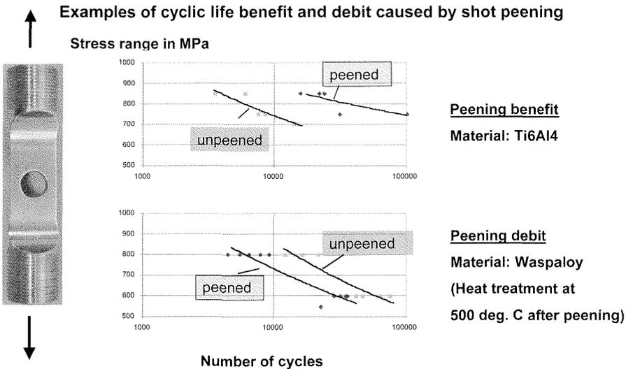
Figure 8: Examples of benefit and debit of fatigue lives produced by shot peening
