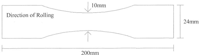
**Figure 1:** Hourglass specimen for corrosion fatigue testing
