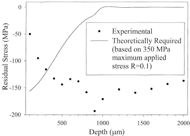
**Figure 5:** Distribution of residual stresses, measured vs theoretically required
