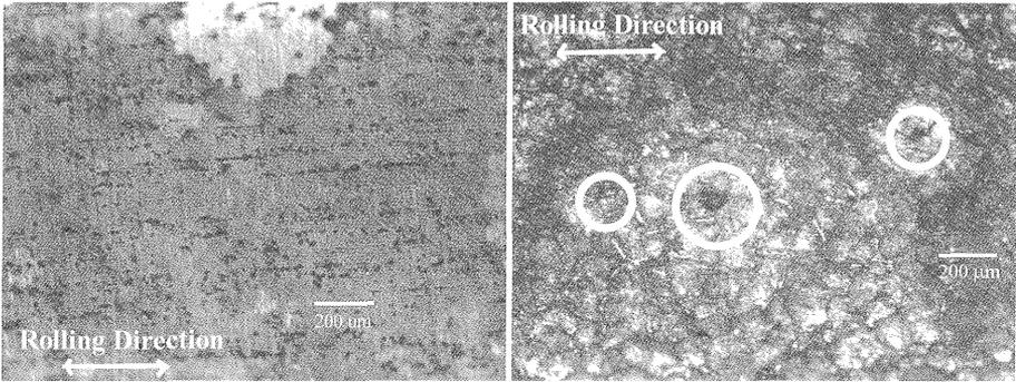
**Figure 4a:** Unpeened – showing strings of pits in the rolling direction
