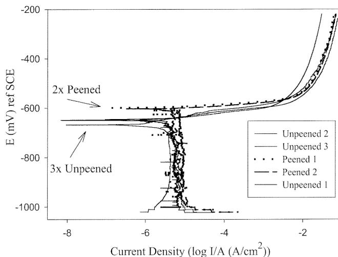
**Figure 3:** Potentiodynamic polarisation plot indicating the difference in  $E_{\text{corr}}$
