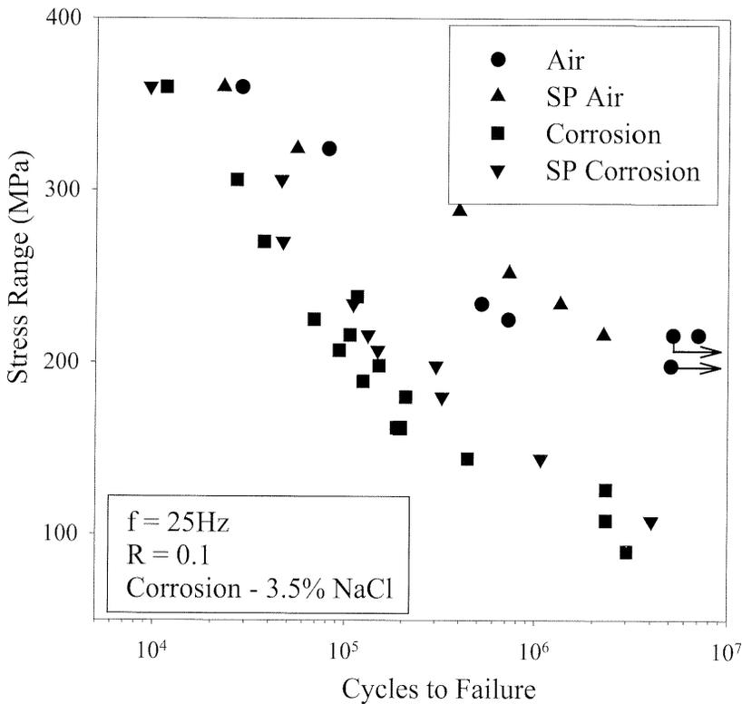
**Figure 2:** Results of air and corrosion fatigue tests
