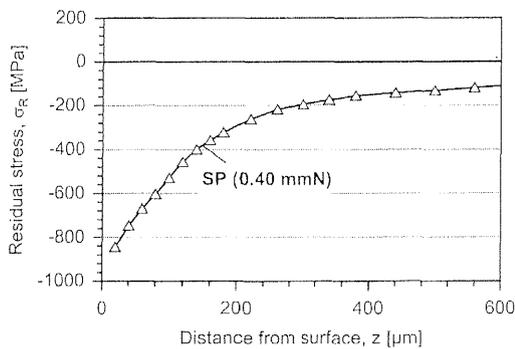
**Figure 9:** Residual stress profile after shot peening (0.40 mmN)
