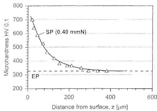
**Figure 8:** Microhardness profile after shot peening (0.40 mmN)
