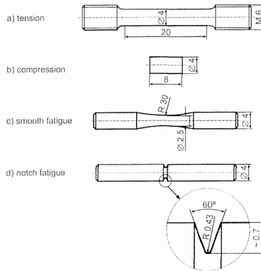
Figure 2: Specimen geometries for mechanical testing
