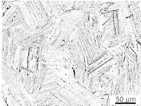
Figure 3: Microstructure of  $\gamma$ (TiAl)
