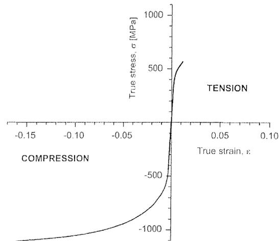
Figure 4: Stress strain curves
