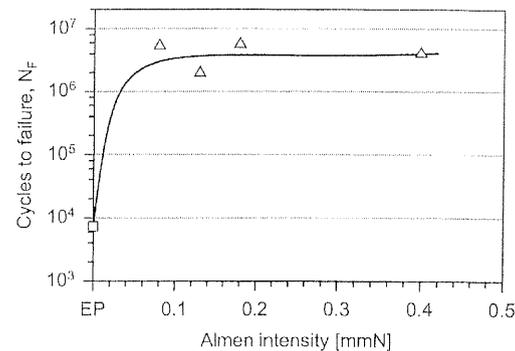
Figure 6: Fatigue life ( $\sigma_a = 700$  MPa) vs. Almen intensity
