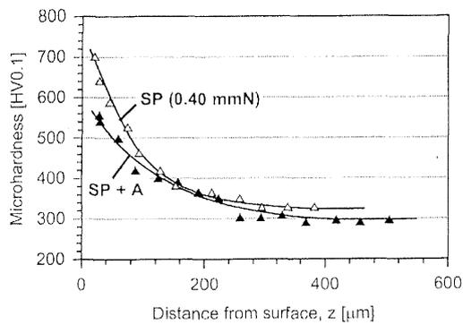
**Figure 13:** Microhardness profile (0.40 mmN), effect of annealing
