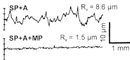
**Figure 17:** Roughness of shot peened and annealed conditions, effect of mechanical polishing (15  $\mu\text{m}$  removed from as-peened surface)
