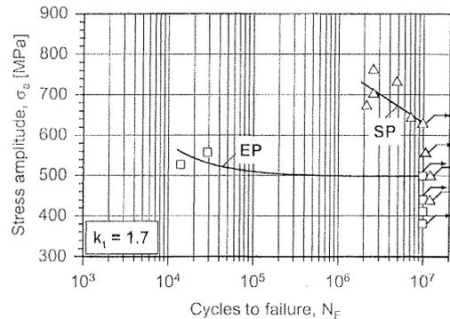
**Figure 12:** S-N curves ( $R = -1$ ) of notched specimens
