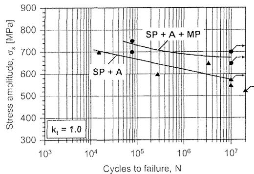
**Figure 18:** S-N curves ( $R = -1$ ) of shot peened and annealed conditions, effect of mechanical polishing (15  $\mu\text{m}$  removed from as-peened surface)
