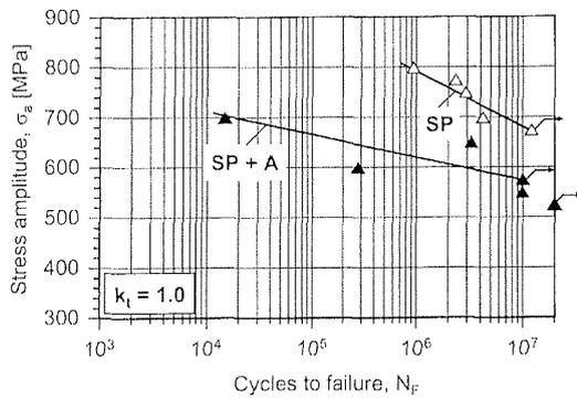
**Figure 15:** S-N curves ( $R = -1$ ) of smooth shot peened specimens, effect of annealing
