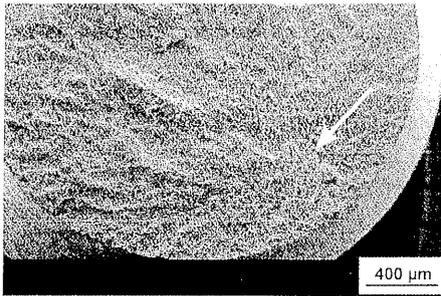
**Figure 11:** Fatigue crack nucleation site in smooth shot peened specimens
