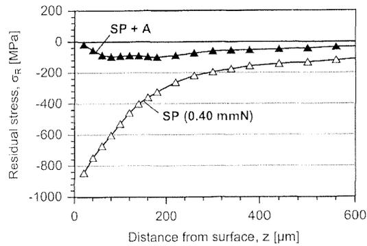
**Figure 14:** Residual stress profile (0.40 mmN), effect of annealing
