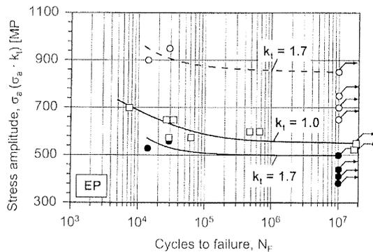
Figure 5: S-N curves in rotating beam loading ( $R = -1$ ), EP
