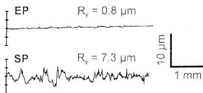
**Figure 7:** Surface roughness profiles (EP-electropolished, SP-shot peened, 0.40 mmN)
