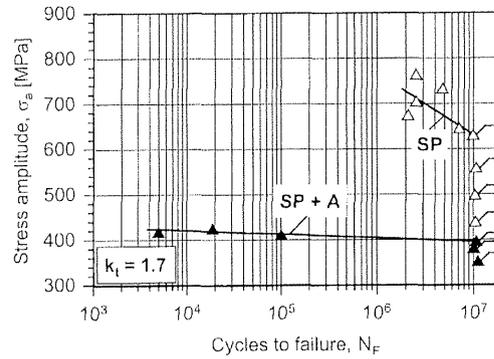
**Figure 16:** S-N curves ( $R = -1$ ) of notched shot peened specimens, effect of annealing
