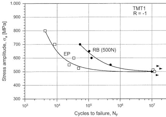
**Figure 10:** S-N curves of KS 120 after optimum roller-burnishing (rotating beam loading in air)
