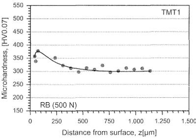
**Figure 8:** Microhardness-depth profile of KS 120 after roller-burnishing
