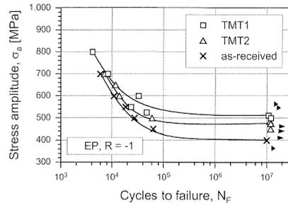
**Figure 4:** S-N curves of KS 120 (rotating beam loading in air)
