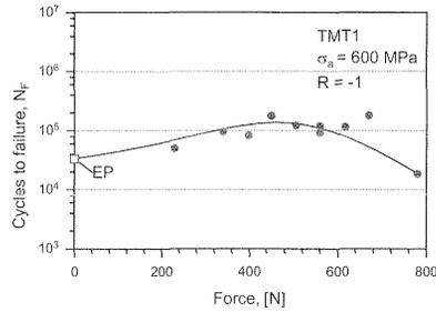
**Figure 9:** Fatigue life ( $\sigma_a = 600$  MPa) vs. rolling force
