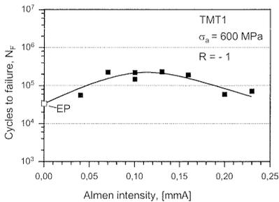
Figure 6: Fatigue life ( $\sigma_a = 600$  MPa) vs. Almen intensity
