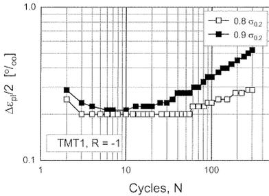
**Figure 3:** Cyclic deformation behavior ( $R = -1$ ) of KS 120
