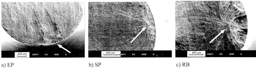
**Figure 11:** Fracture surfaces of fatigue failed KS 120 specimens, TMT1 (arrow indicates crack nucleation site)
