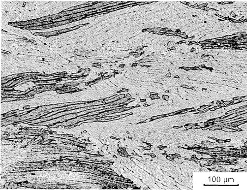
**Figure 1:** Microstructure of as-received KS120
