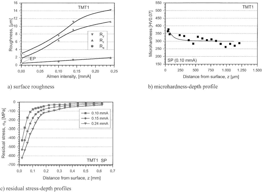
Figure 5: Surface properties of KS 120 after shot peening
