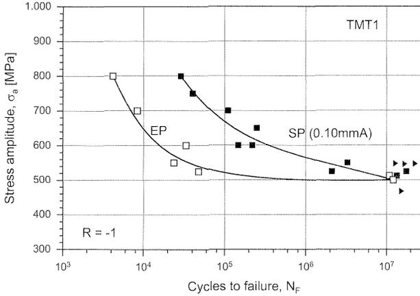
**Figure 7:** S-N curves of KS 120 after optimum shot peening (rotating beam loading in air)
