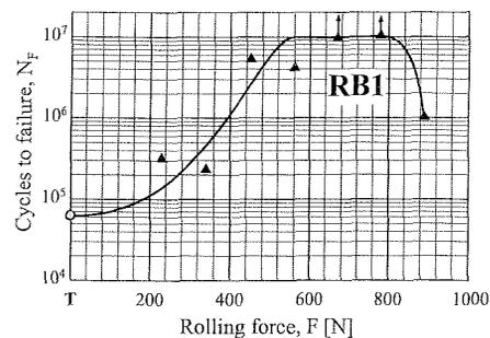
**Figure 11:** Fatigue life ( $\sigma_a = 700$  MPa) of RB1 condition
