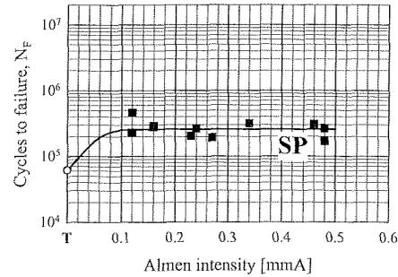
**Figure 9:** Fatigue life ( $\sigma_a = 700$  MPa) of SP condition
