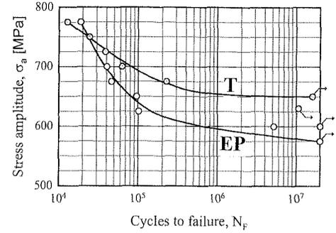
**Figure 5:** S-N curves in rotating beam loading of reference conditions T and EP
