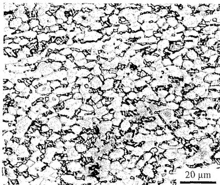
Figure 1: Microstructure of Ti-6Al-4V
