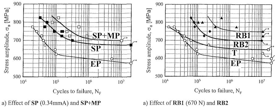
**Figure 12:** S-N curves in rotating beam loading of the various surface treated conditions in Ti-6Al-4V
