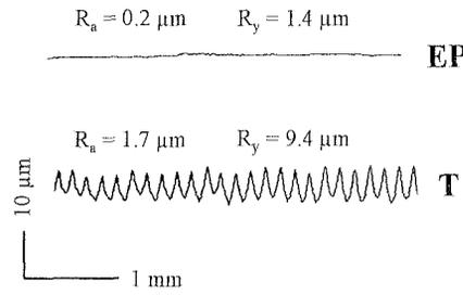
**Figure 4:** Roughness profiles of reference conditions T and EP
