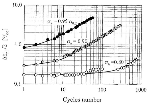
Figure 3: Cyclic deformation characteristics in Ti-6Al-4V ( $R = -1$ )
