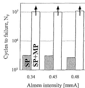
**Figure 10:** Fatigue life ( $\sigma_a = 700$  MPa) of SP condition after mechanical polishing SP+MP
