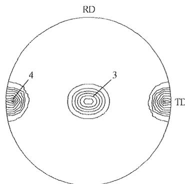
Figure 2: (0002) pole figure of Ti-6Al-4V
