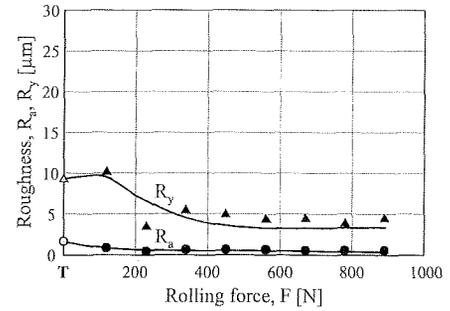
**Figure 7:** Surface roughness vs. rolling force (RB1)
