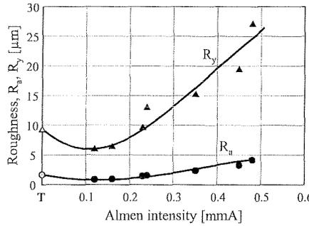
**Figure 6:** Surface roughness vs. Almen intensity (SP)
