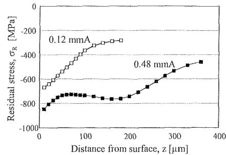
**Figure 8:** Residual stress-depth profiles after shot peening (SP)
