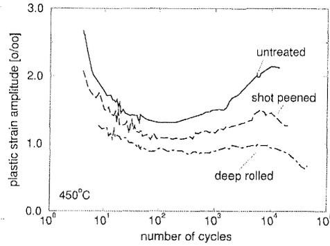
**Figure 2:** Cyclic deformation at 450 °C ( $\sigma_a = 200$  MPa,  $R = -1$ ,  $f = 5$  Hz)
