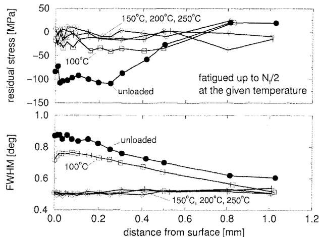
**Figure 4:** Relaxation of near surface residual stresses and FWHMs in deep rolled magnesium alloy AZ31 (rolling pressure 100 bar) after stress-controlled fatigue at temperatures from 100 to 300 °C ( $\sigma_a = 75$  MPa,  $R = -1$ ,  $f = 5$  Hz,  $N_f/2$  cycles ( $N_f =$  cycles to failure)).
