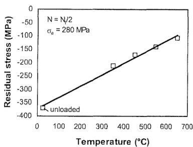
**Figure 6:** Surface residual stresses of deep rolled AISI 304 (rolling pressure 150 bar) before and after stress-controlled high temperature fatigue at different temperatures ( $\sigma_a = 280$  MPa,  $R = -1$ ,  $f = 5$  Hz,  $N = N_f/2$ )
