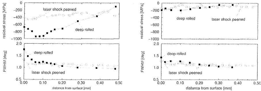
**Figure 5:** Near surface residual stress and FWHM-depth profiles of deep rolled (rolling pressure 150 bar) and of laser shock peened (peening intensity 7 GW/cm<sup>2</sup>, coverage 200 %) Ti-6Al-4V before (left) and after (right) high temperature fatigue ( $\sigma_a = 460$  MPa,  $R = -1$ ,  $f = 5$  Hz,  $N = N_f/2$ )
