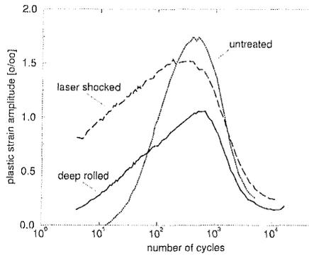
**Figure 1:** Cyclic deformation behavior of Ti-6Al-4V at behavior of AISI 304 450 °C ( $\sigma_a = 460$  MPa,  $R = -1$ ,  $f = 5$  Hz)
