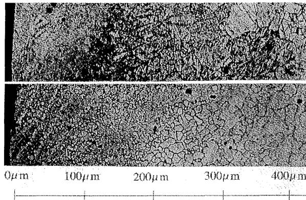
**Figure 9:** Near-surface microstructure of deep rolled AZ31 before (above) and after (below) high thermal exposure (300 °C, 10 seconds)
