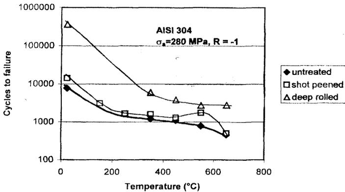
**Figure 3:** Stress controlled fatigue lifetimes of AISI 304 in different surface treatment states for temperatures from room temperature to 650 °C ( $\sigma_a = 280$  MPa,  $R = -1$ ,  $f = 5$  Hz)
