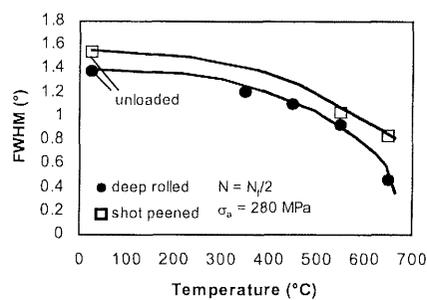
**Figure 7:** Surface FWHM-values of deep rolled and of shot peened (peening intensity 0.120 mmA) AISI 304 before and after stress-controlled fatigue at different temperatures ( $\sigma_a = 280$  MPa,  $R = -1$ ,  $f = 5$  Hz,  $N = N_f/2$ )
