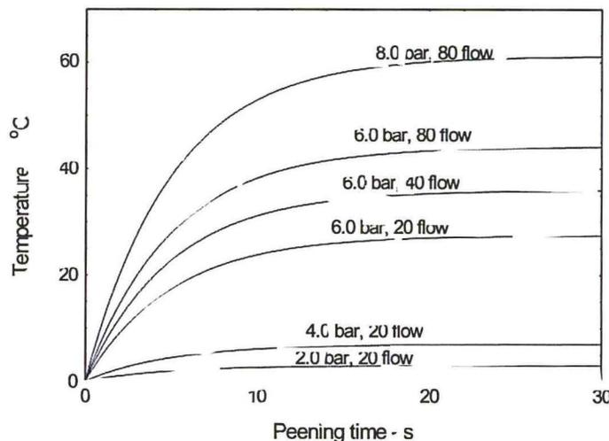
Fig. 3 Heating curves for N strip during peening using S170 shot
