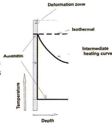
Fig. 2 Adiabatic, intermediate and isothermal heating curves
