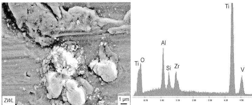
**Figure 3:** SEM photograph of residual particles at the shot peened surface (left) and EDX verification of zirconia contamination (right).
