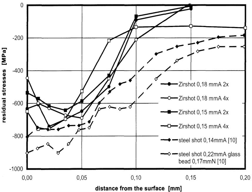
**Figure 2:** Residual stress states of TiAl6V4 rods after shot peening with Zirshot in comparison with TiAl6Nb7 rods after shot peening with steel shot.
