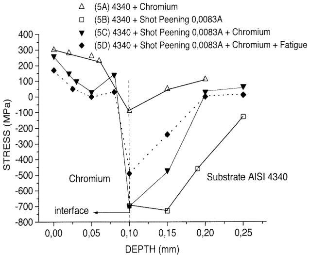
Figure 5 - Residual stress fields with 39HRC.
