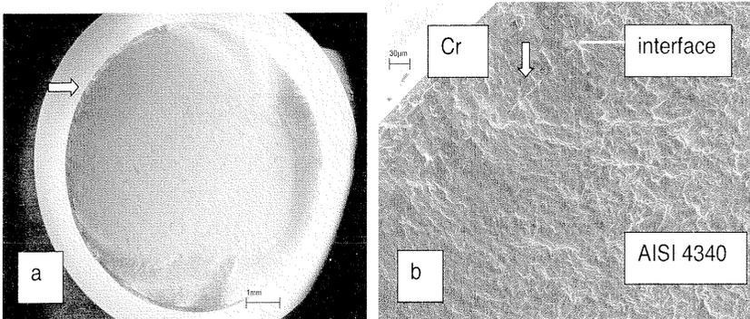
Figure 6 – a) An overview of the fatigue fracture surface: base material with chromium plating (53HRC); b) Detail of crack source.
