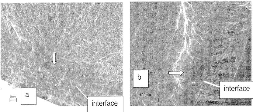
Figure 7 –Fatigue fracture surfaces: base material with shot peening and chromium plating a) 53HRC b) 39HRC.
