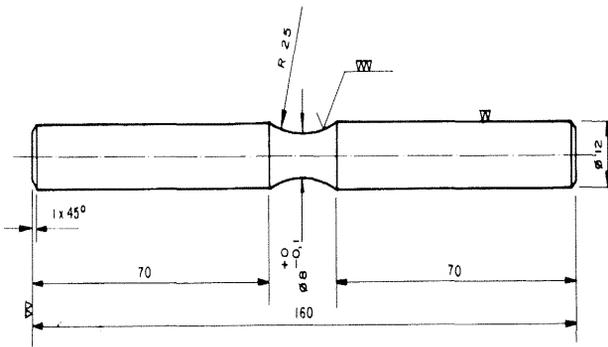
Figure 1 – Rotating bending fatigue test specimen.
