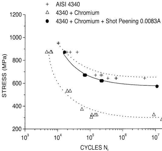
Figure 3 – Fatigue results of AISI 4340 with 39HRC.
