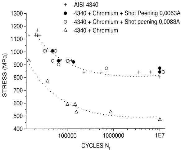
Figure 2 – Fatigue results of AISI 4340 with 53HRC.
