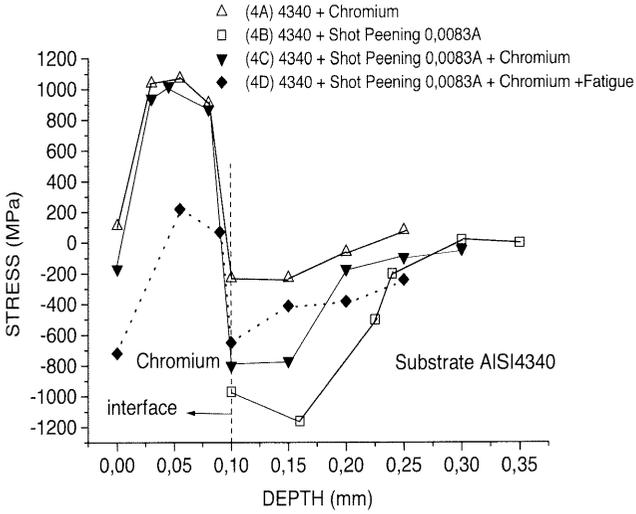
Figure 4 – Residual stress fields with 53HRC.
