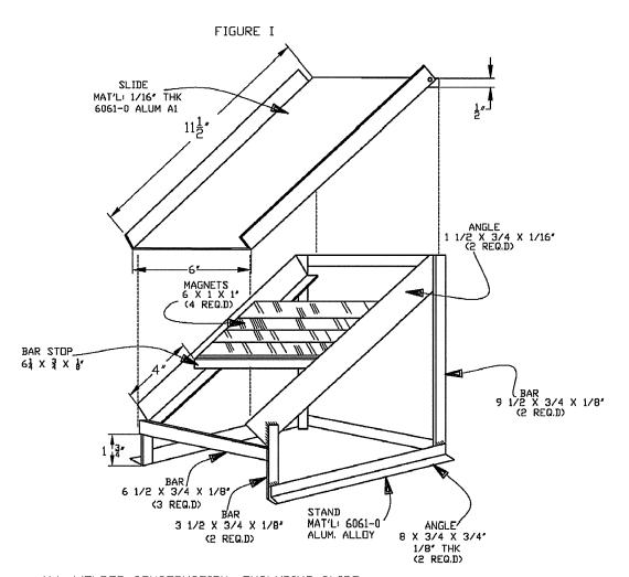
ALL WELDED CONSTRUCTION....EXCLUDING SLIDE MAGNETS MUST BE MINIMUM 10,000 GAUSS STRENGTH
