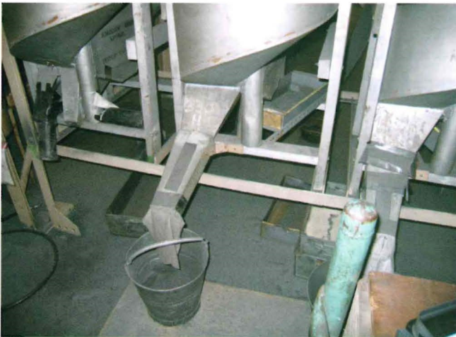
Fig.12 Segregation of acceptable and rejected shot fractions.
