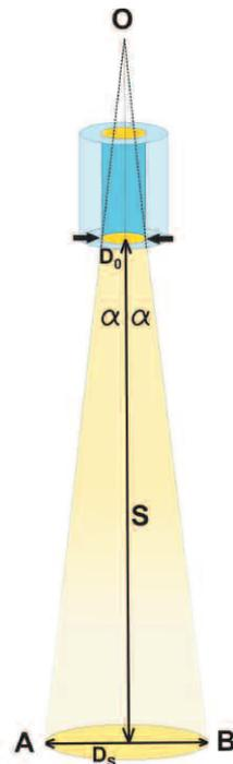
Fig.3. Geometry of an inbound conical shot stream.
