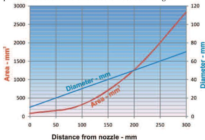
Fig.4 Variation of cone diameter and cross-sectional area with distance from a 10mm diameter,  $5.7^\circ$ , nozzle.
