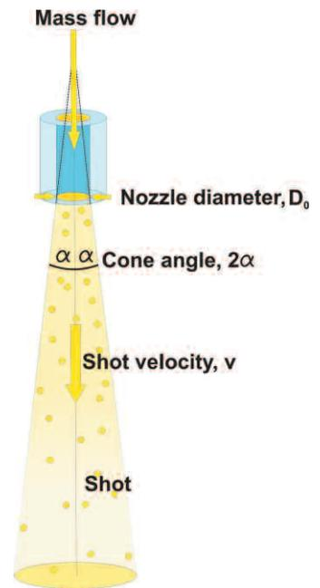
Fig.2. Primary parameters of inbound shot stream - shown as a truncated right circular cone.
