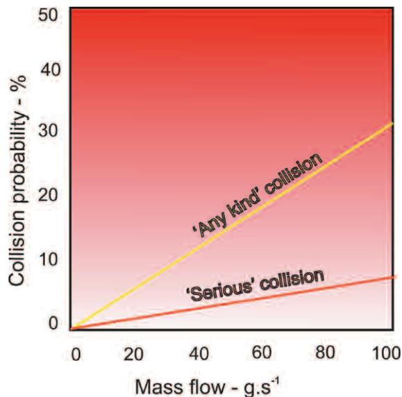
Fig.11 Effect of mass flow on collision probabilities – for specified shot stream parameters.
