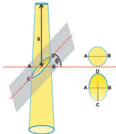
Fig.6. Ellipse formed by flat surface intersecting a circular cone at an angle  $\theta$ .
