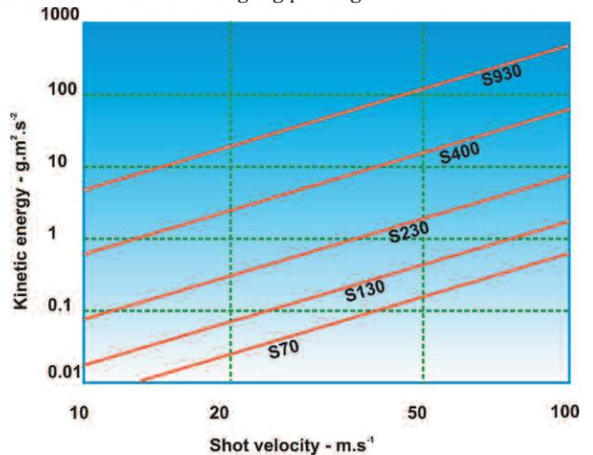
Fig.8. Variation of kinetic energy with size and velocity of cast steel shot particles.
