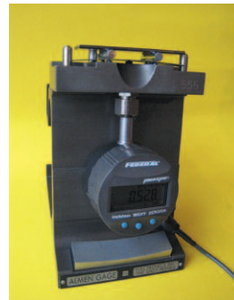
Fig.21. Raft device for holding paramagnetic specimens on a magnetic hold-down Almen gage.
