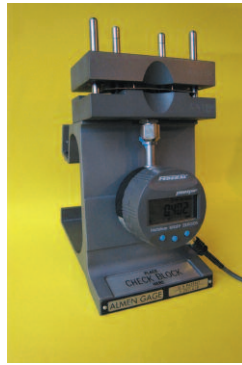
Fig.9 Photograph showing pin hold-down mechanism used for Almen Aero gage TSP-3AA.
