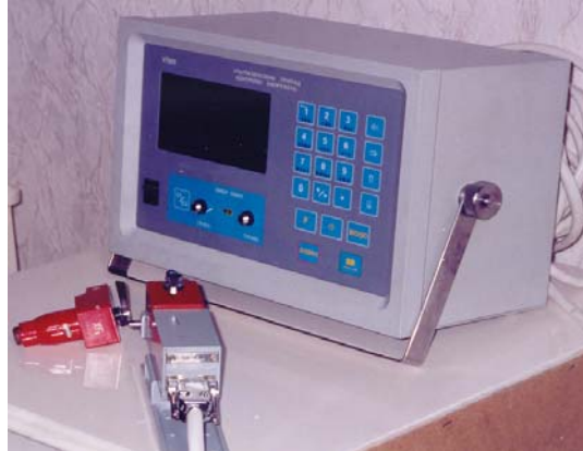
Figure 2. Portable Residual Stress Measurement System. Shown with two gages.
