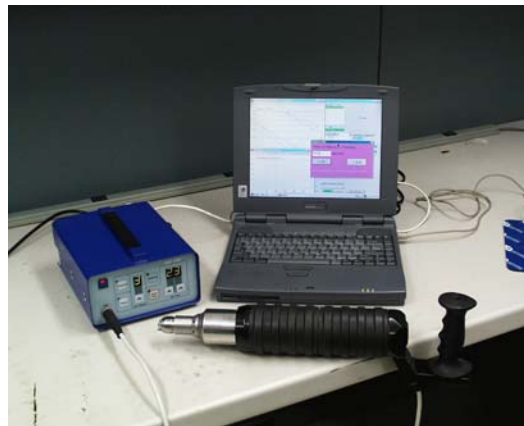
Figure 1. Computerized Complex for Ultrasonic Peening of parts and welded elements
