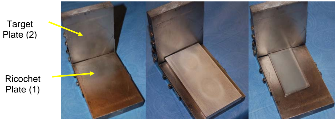
Figure 4: Tool Steel, Aluminum, and Mild Steel Ricochet Surfaces
