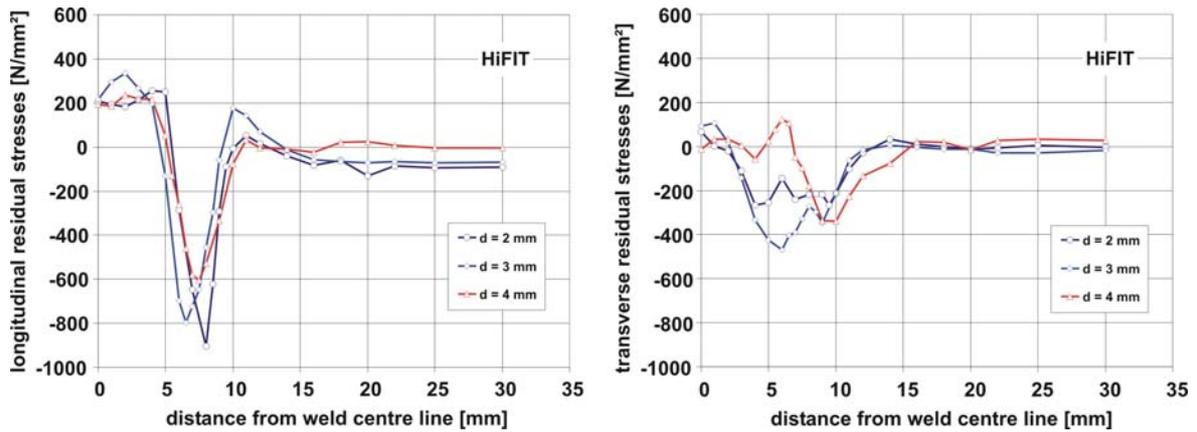
Fig 7: Residual stress profiles around the treated weld toe of double-V-welds after hammer peening with different pin diameters (HiFIT).
