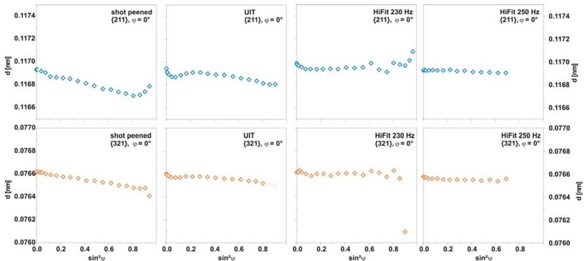
Figure 10:  $d$ - $\sin^2\psi$ -distributions of mechanically treated samples measured with synchrotron radiation.
