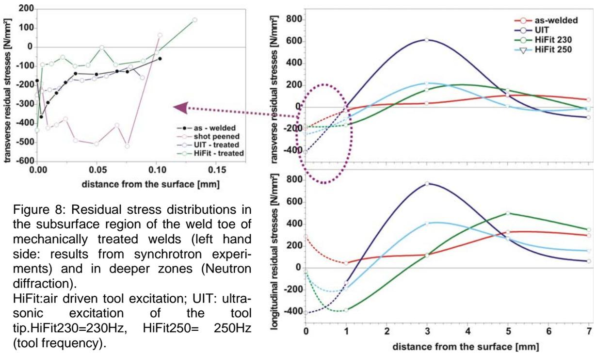
Figure 8: Residual stress distributions in the subsurface region of the weld toe of mechanically treated welds (left hand side: results from synchrotron experiments) and in deeper zones (Neutron diffraction). HiFit: air driven tool excitation; UIT: ultrasonic excitation of the tool tip. HiFit230=230Hz, HiFit250= 250Hz (tool frequency).
