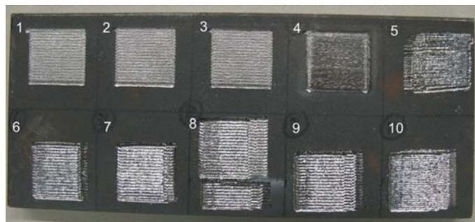
Fig 4: Base metal specimen with hammer peening track generated with different methods and intensities.
