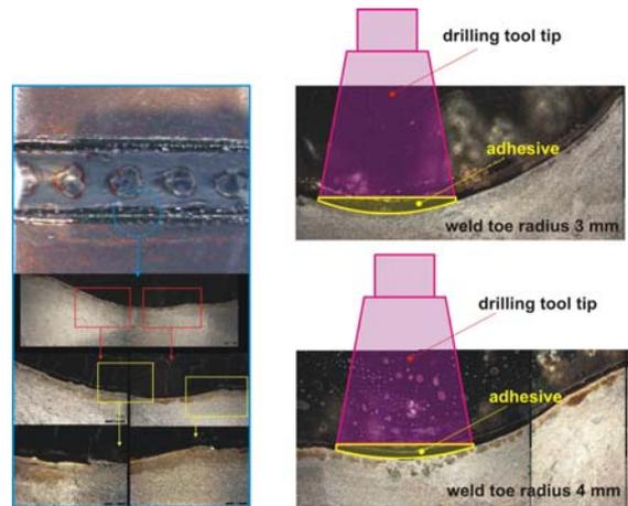
Figure 2: Geometrical shape of the weld toe after different local hammer peening procedures and resulting systematic barriers for hole drilling measurements.
