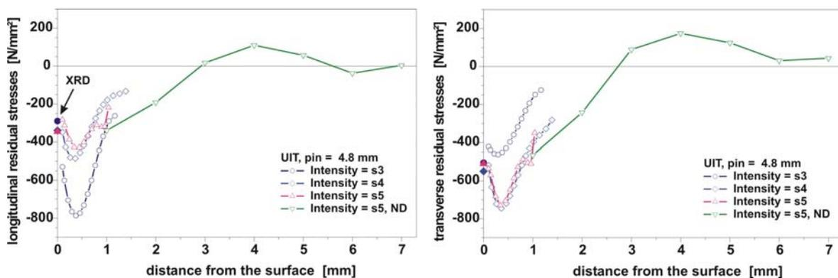
Fig 6: Residual stress depth profiles in UIT-treated fields in the base material S690. Treatment was performed with different intensities. XRD: X-ray diffraction, ND: Neutron diffraction, rest: Hole drilling method. (s3...s5 is a device specific intensity (e.g.tool amplitude) indicator which is not explained more detailed by the manufacturer of the device, s1 is the lowest, s5 the highest possible intensity).
