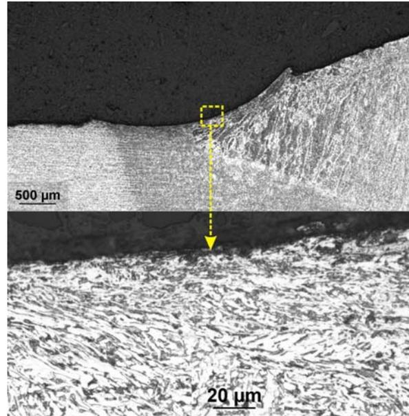
Figure 10: shape of a UIT-track and oriented grain structure in the centre of the track surface.
