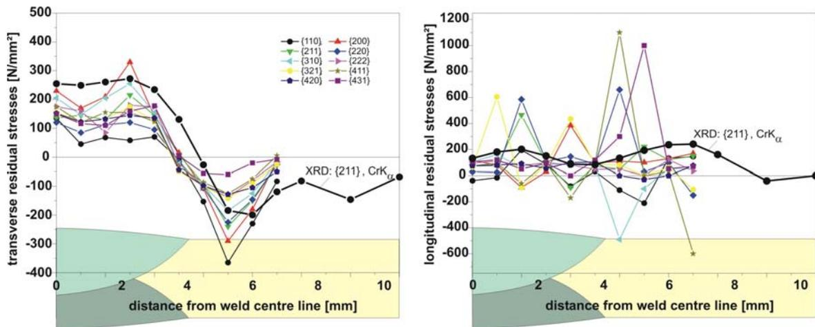
Figure 9: Residual stress distributions from energy dispersive measurements in a TIG-welded sample of the structural steel S355J2G3. Calculations from different lattice planes in comparison to measurements with help of X-ray diffraction. Left hand side: transverse residual stresses, right hand side: longitudinal residual stresses
