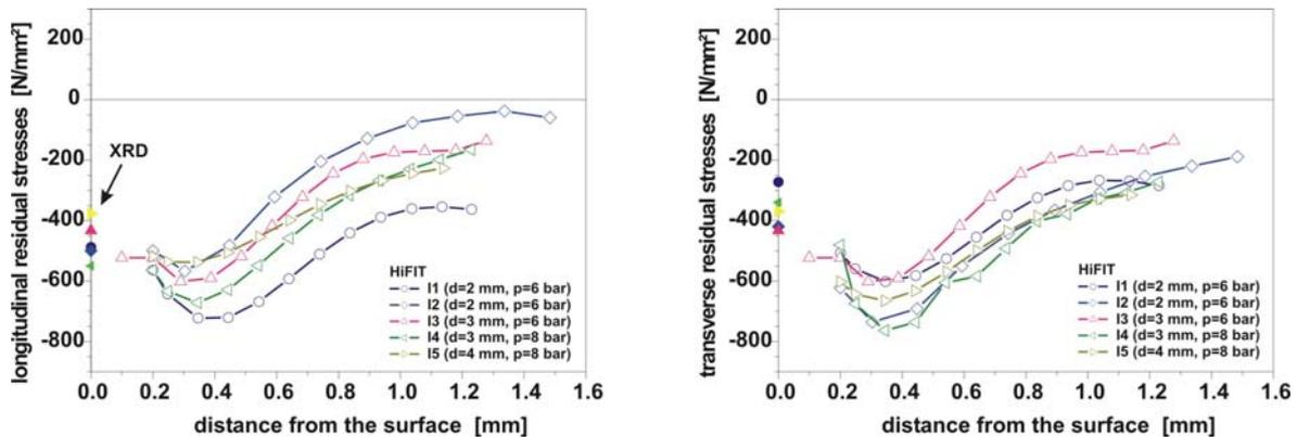
Fig 5: Residual stress depth profiles in HiFIT-treated fields in the base material S690. Treatment was performed with different intensities. (p [bar] is the excitation pressure of the air driven tool).
