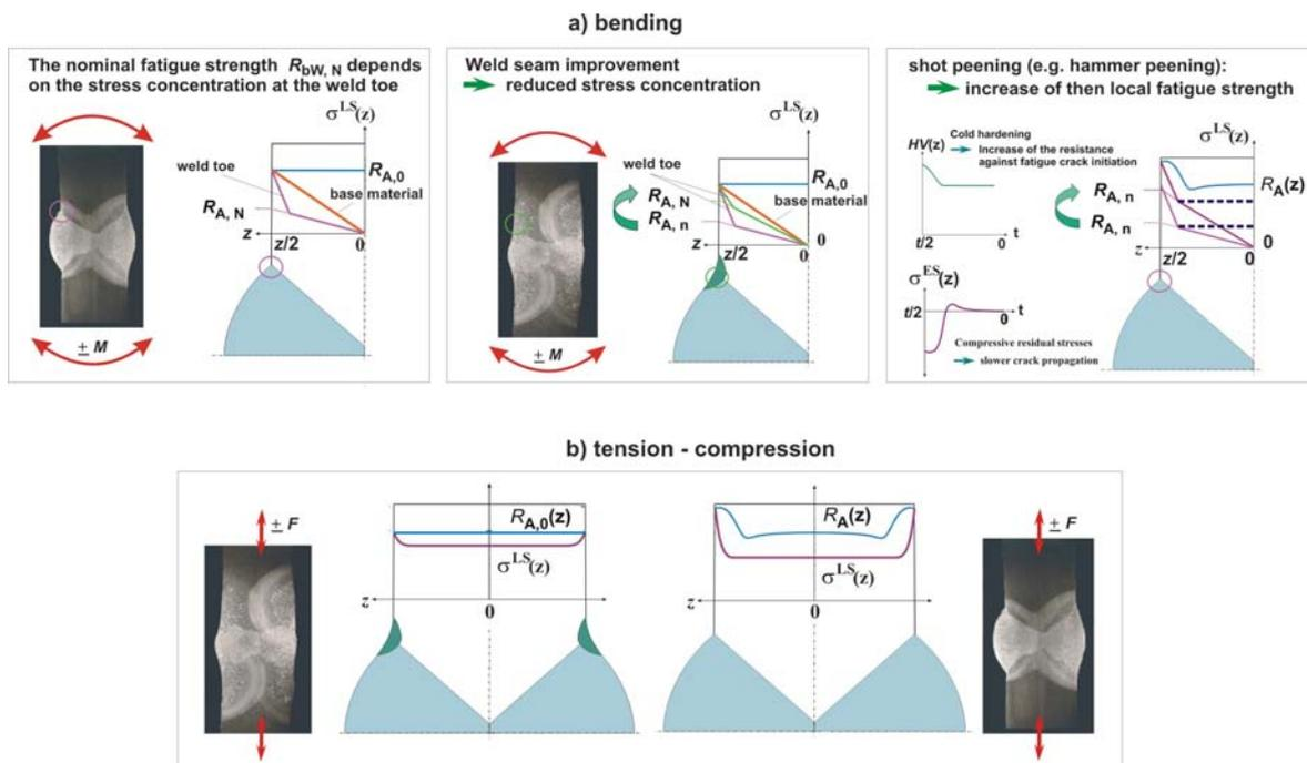
Figure 1: Schematical representation of the influence of compressive residual stresses and cold hardening due to mechanical surface treatments on the local fatigue strength of welded joints.
