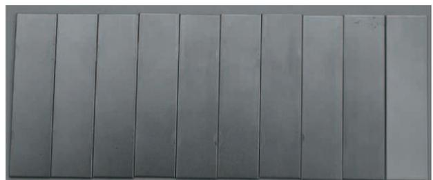
Fig.12. Digital optical photograph of a set of Almen strips peened after pre-polishing.
