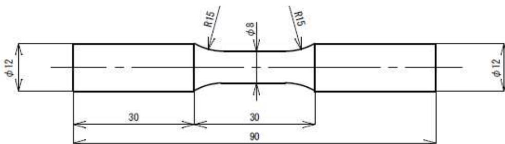
(b) Specimens of AC8AH and AM60B
