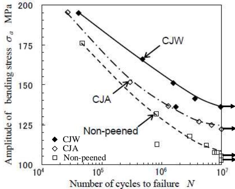
Fig. 5 Improvement of fatigue strength of aluminum alloy AC8AH by cavitation peening
