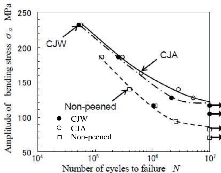
Fig. 4 Improvement of fatigue strength of aluminum alloy AC4CH by cavitation peening
