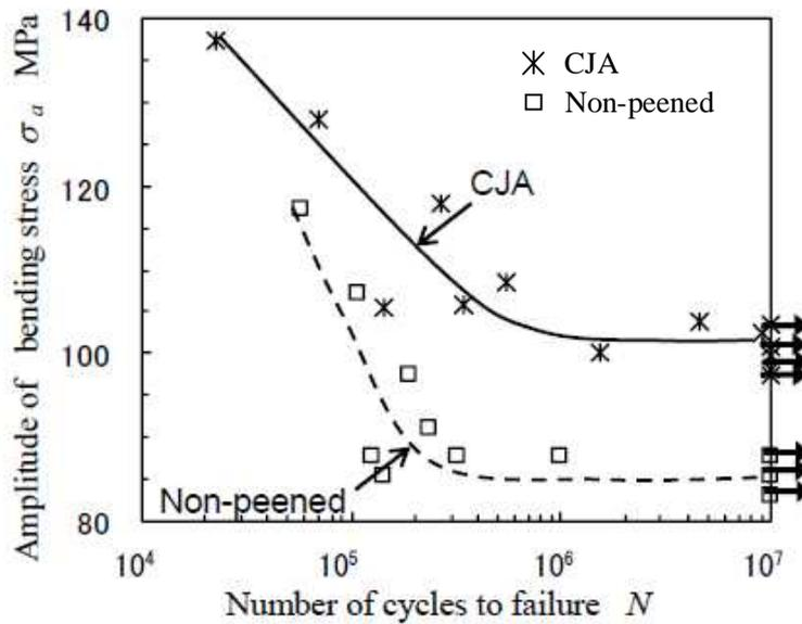
Fig. 3 Improvement of fatigue strength of magnesium alloy AM60B by cavitation peening
