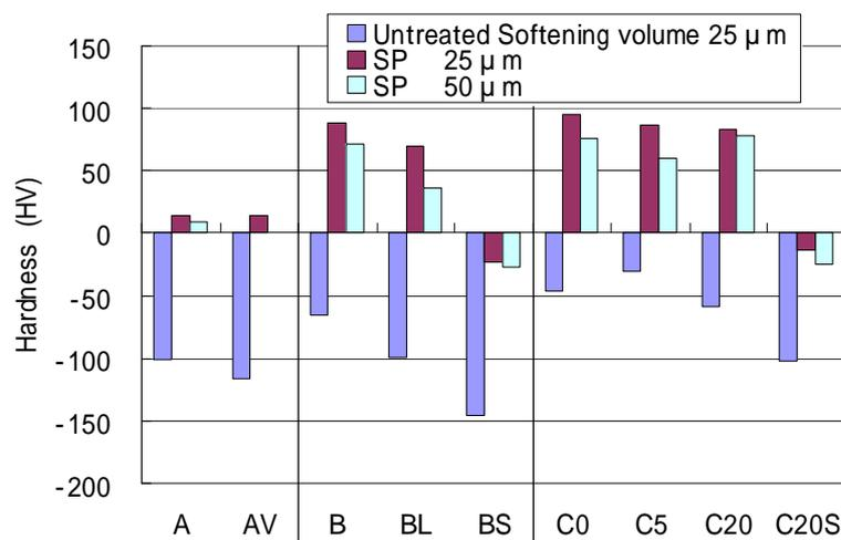
Figure 4 Closs section hardness after SP
