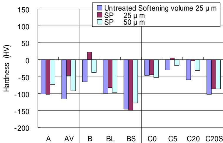
Figure 5 Cross section hardness after SP
