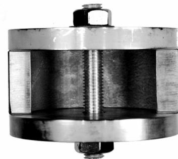
Fig. 2 Bolt-type specimen set in the special fixtures.
