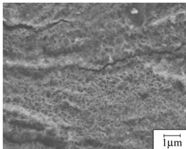
Fig. 3. SEM micrograph of SUYP-1 specimen with lamellar structure after FPB treatment (Condition A).
