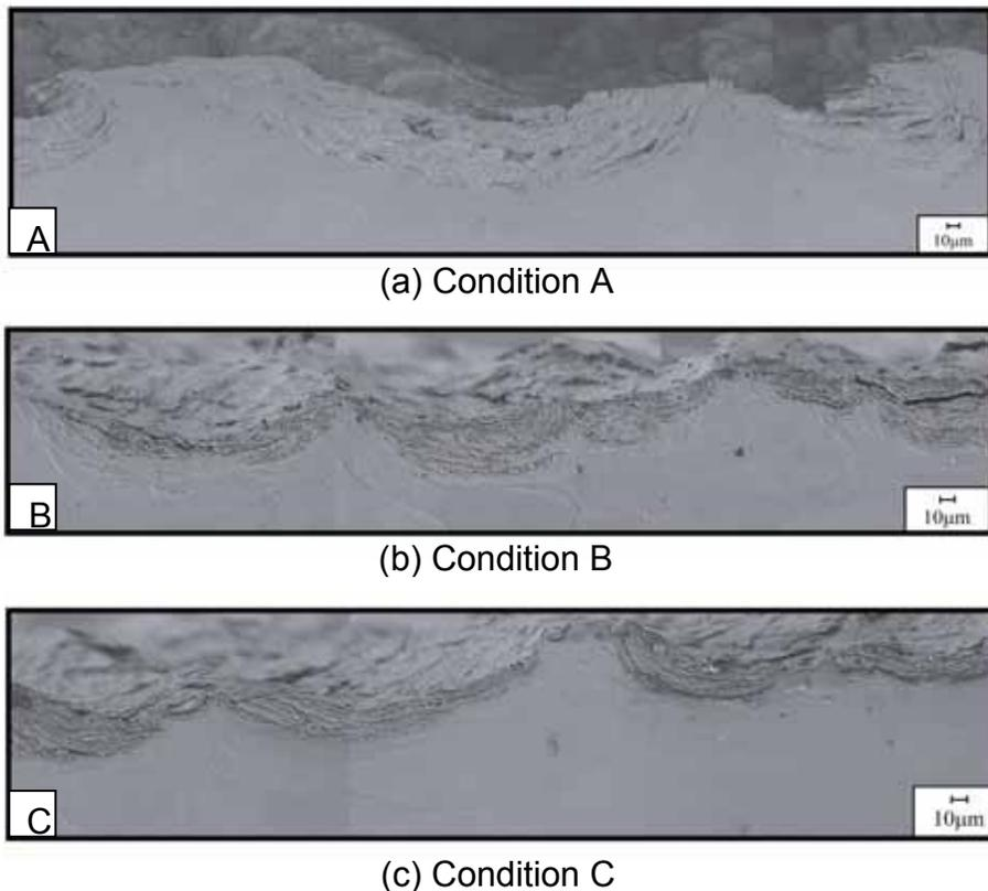
Fig. 2. SEM micrographs of SUYP-1 specimen for various FPB consitions.
