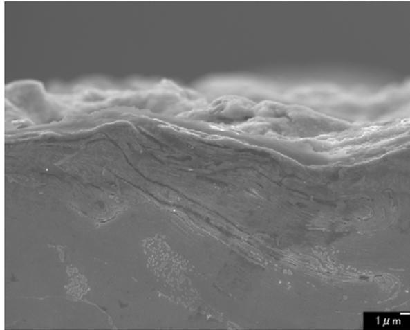
Fig. 4. SEM micrograph of SS400 specimen with lamellar structure after FPB treatment (Condition A).
