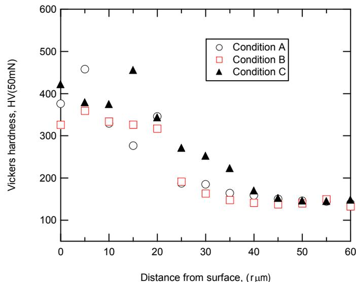
Fig. 5. Hardness distribution of SUYP-1 for various conditions.
