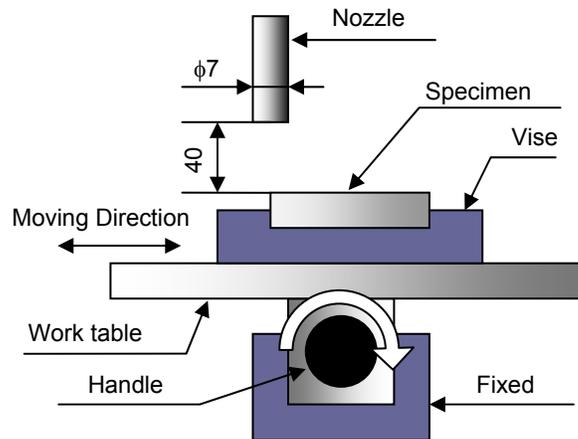
Fig. 1. Schematic of FPB processing.
