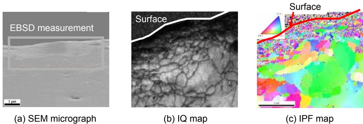
Fig. 6. EBSD measurements for SUYP-1 after FPB treatment.
