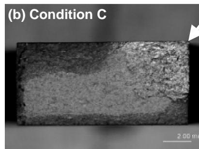
Fig. 3 Fatigue fracture surface of laser peened coupon specimens
