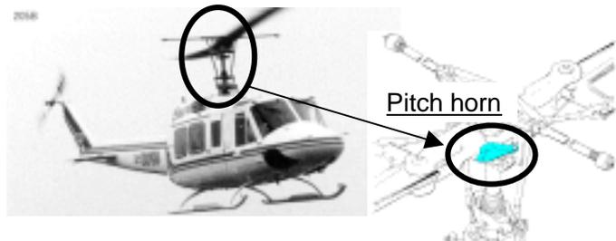
Fig. 6 Pitch horn of helicopter
