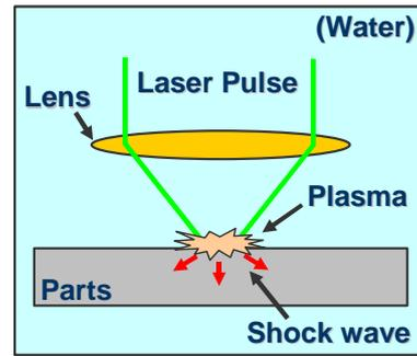
Fig.1 Schematic of laser peening
