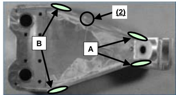
(b) Laser peened test specimen
