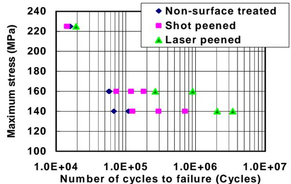
Fig. 5 Result of notched fatigue tests
