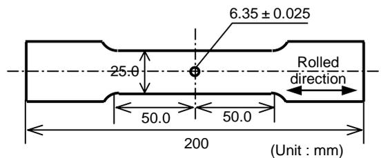
Fig. 4 Notched coupon specimen (Thickness: 6mm)
