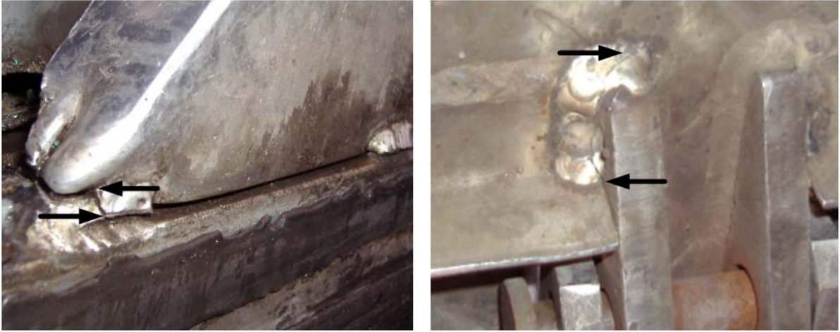
Fig. 1 Fatigue fracture in the step of rolling stock due to repeated load.
