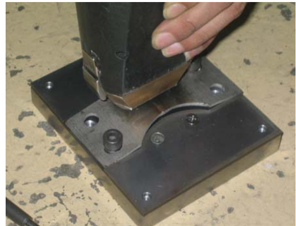
Fig. 3 Ultrasonic peening process
