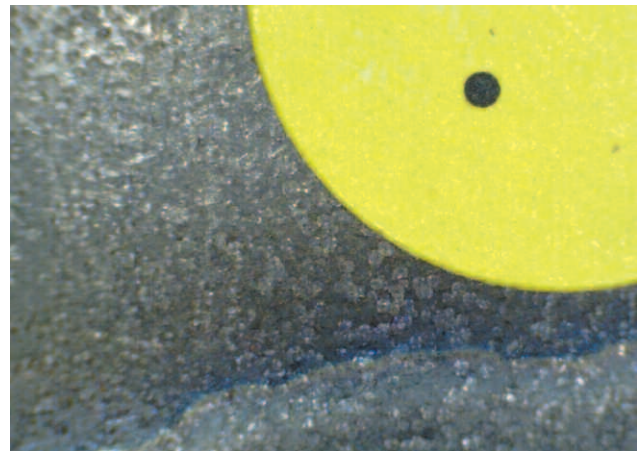
Fig.11 Decal black dot on self-adhesive yellow label stuck to peened component.
