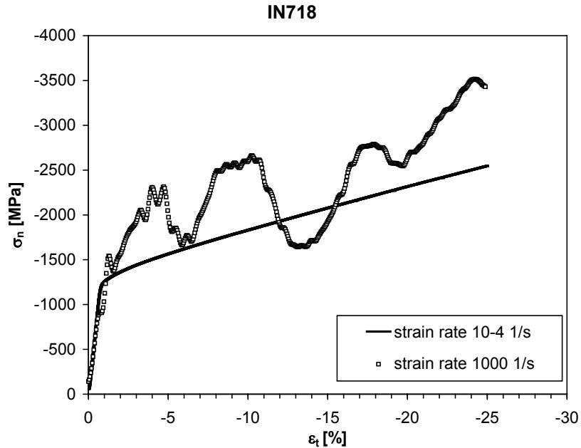
**Figure 2:** Typical measured compressive stress strain curve for the two different strain rates ( $\dot{\varepsilon}_t = 10^{-4} \text{ 1/s}$  and  $1000 \text{ 1/s}$ ) for IN718
