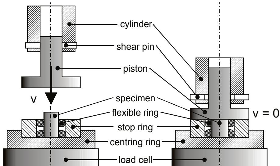
**Figure 1:** Schematic diagram of the testing device of the high strain rates
