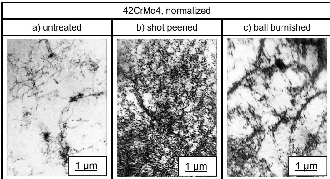
**Figure 5:** Transmission electron micrograph at surface distance of 0.08 mm in a untreated (a), a shotpeened (b) and a ball burnished (c) normalized AISI4140 specimen [4]
