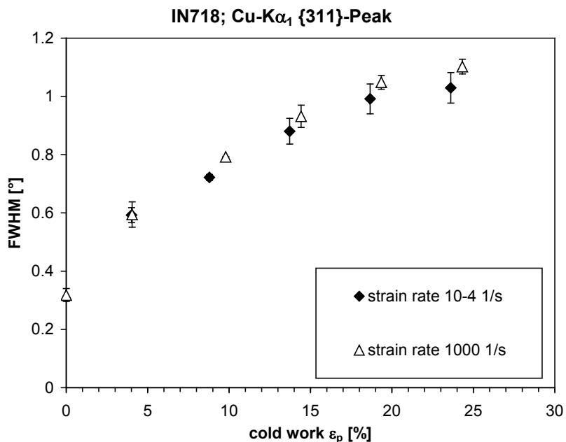
**Figure 3:** FWHM measured after different loadings for IN718
