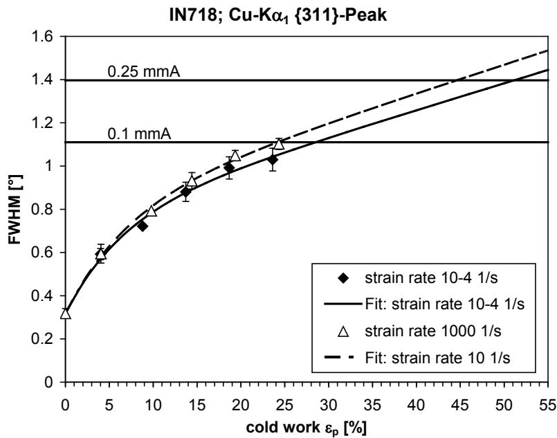
**Figure 4:** FWHM measured after shot peening and different loadings and for the different strain rates fitted with equation (2) for IN718
