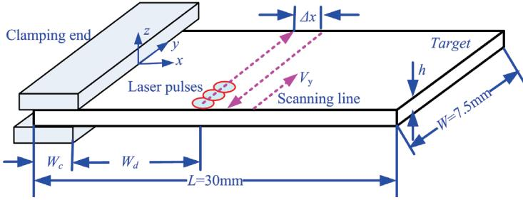
Fig.3 Configuration of specimens irradiated by laser pulses
