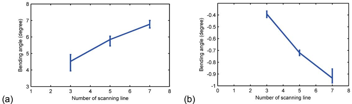
Fig.4 The effect of scanning-line number on the bending,  $I_p=3.85$  GW/cm $^2$ ,  $\Phi D = 1.2$ mm,  $V_y=720$ mm/min : (a) 0.5mm thick target; (b) 2mm thick target
