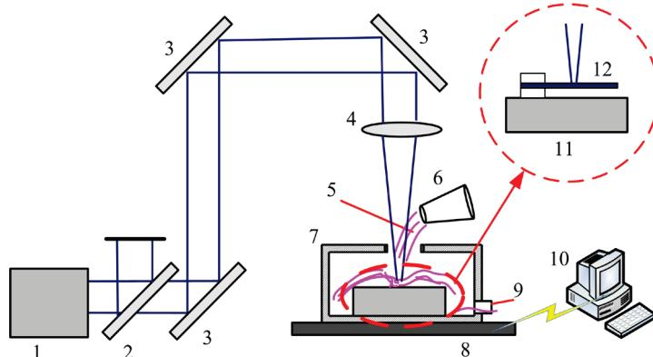
Fig.2 Schematic of experimental setup for laser peen forming: 1-Nd:YAG laser, 2-beam splitter, 3-reflecting mirror, 4-lens, 5-water, 6-nozzle, 7-container, 8-X/Y stage, 9-water outlet, 10-computer, 11-sample holder, 12-target
