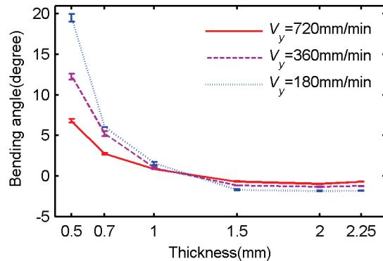
Fig. 7 The effect of scanning velocity on the bending deformation of sheet metal with different thickness,  $\phi D=1.2\text{mm}$ ,  $I_p=3.85\text{GW}/\text{cm}^2$ ,  $N_x=7$
