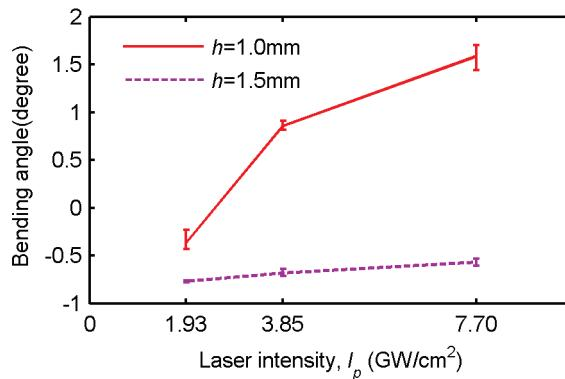
Fig.6 The effect of laser intensity on the bending deformation of sheet metal,  $\Phi D=1.2\text{mm}$ ,  $V_y=720\text{mm/min}$ ,  $N_x=7$
