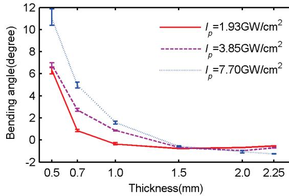
Fig.5 The effect of specimen thickness on the bending deformation of sheet metal with different laser intensities,  $\Phi D = 1.2\text{mm}$ ,  $V_y=720\text{mm/min}$ ,  $N_x=7$
