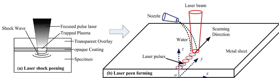
Fig.1 Schematic of the laser peen forming process
