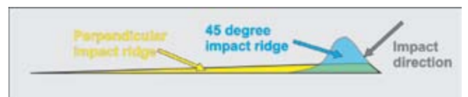
Fig.6. Comparison of perpendicular and 45o dent ridges.
