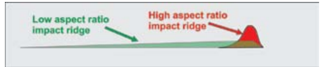
Fig.9 Increase of impact ridge height with increase of indent aspect ratio.
