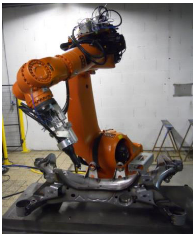
Figure 30 : Robotic UNP on automotive chassis
