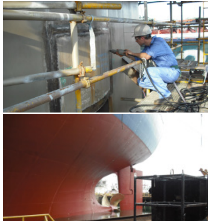
Figure 27 : Nordic Sea Tanker Rudder repair
