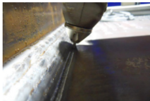
Figure 15 : Ultrasonic needle peening of the weld toe
