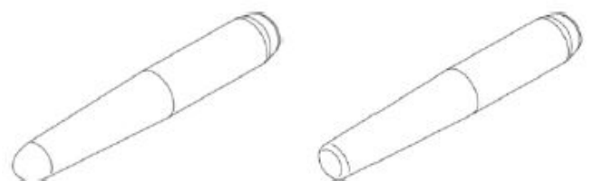
Figure 10 : 1.5 mm radius impactor and 3.00 mm radius impactor (SONATS)
