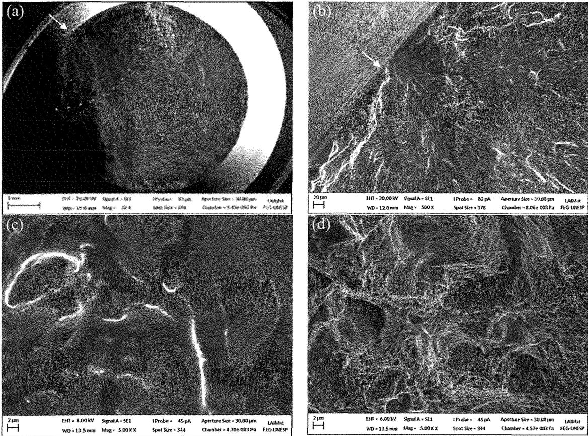
Figure 3. Base material fracture surfaces. R= 0.1. Maximum stress 372.8 MPa
