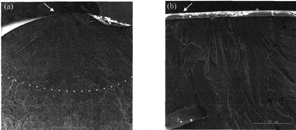
Figure 4. Anodized base material fracture surfaces, R= 0.1. Maximum stress 372.8 MPa.
