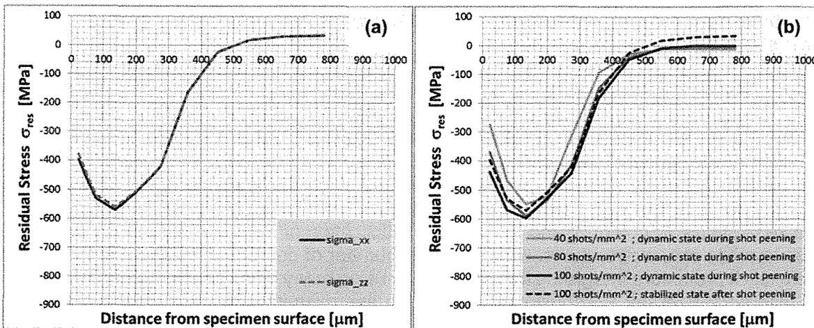
Figure 4: (a) Residual stress depth profiles for longitudinal direction and transverse direction
