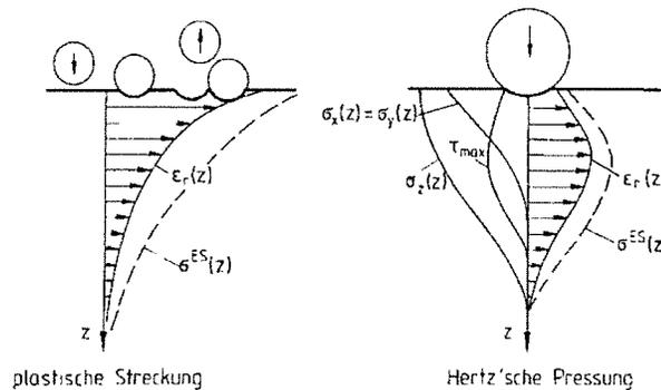
Figure 1: Mechanisms of the development of residual stresses in shot peening [1]: plastic elongation (left), Hertzian pressure (right).
