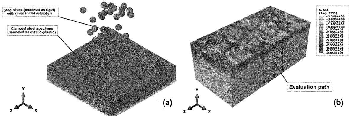
Figure 3: (a) FE-Model of specimen and shots (b) Stress distribution after shot peening (cut view), exemplary evaluation paths
