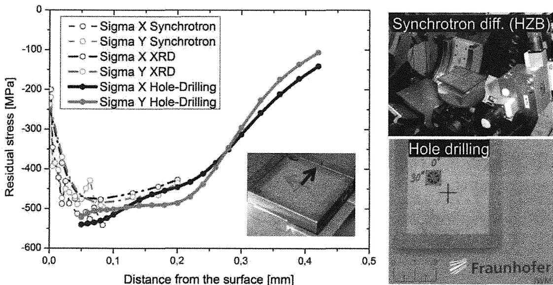
Figure 7: Experimental determination of the residual stress depth profiles in sample C by means of x-ray and synchrotron diffraction and hole drilling method.
