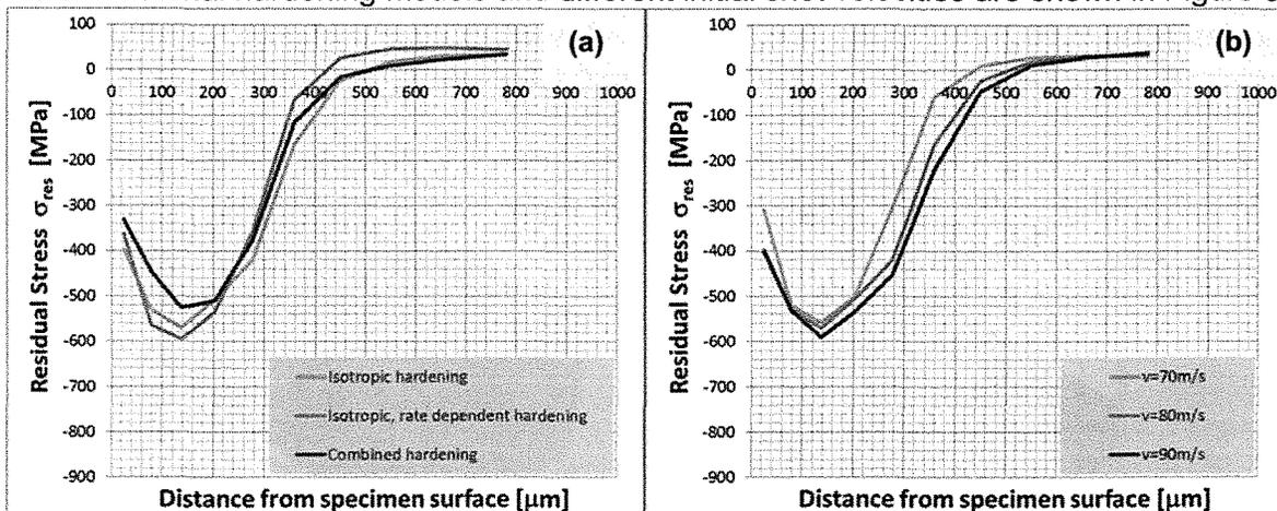
Figure 5: (a) Residual stress depth profiles for different material hardening models (b) Residual stress depth profiles for different initial shot velocities
