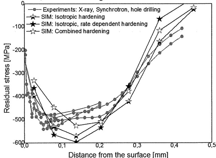
Figure 8: Comparison of the numerical and experimental results.
