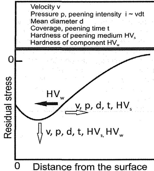
Figure 2: A qualitative model showing the influence of the shot peening parameters on the residual stresses [3].
